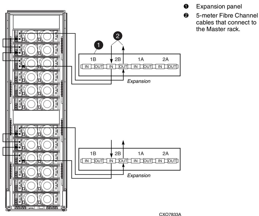
**Figure 4–19: 0C6D + 6D configuration—Fibre Channel loop 2B with expansion panels**
