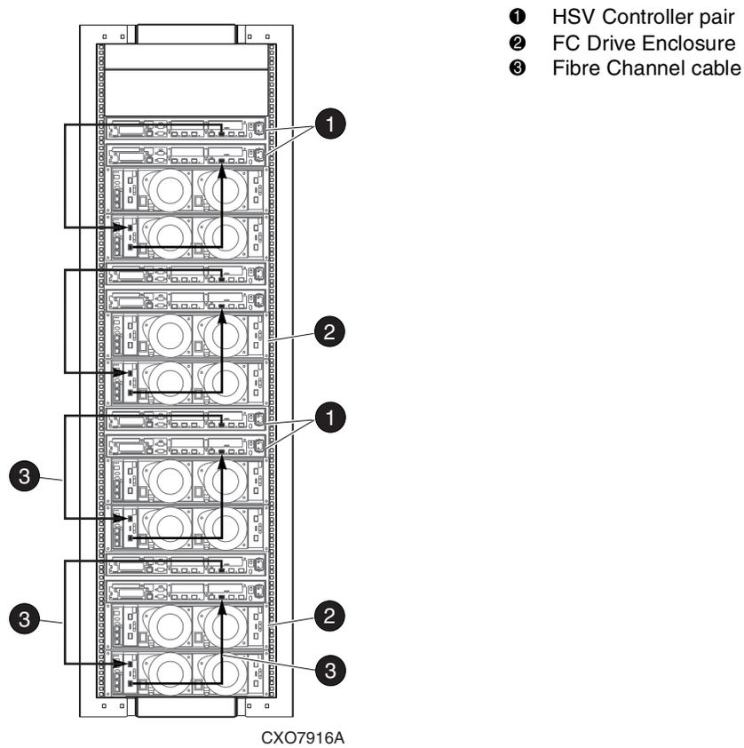
Figure 2–25: 8C8D configuration—Fibre Channel loop 2B
