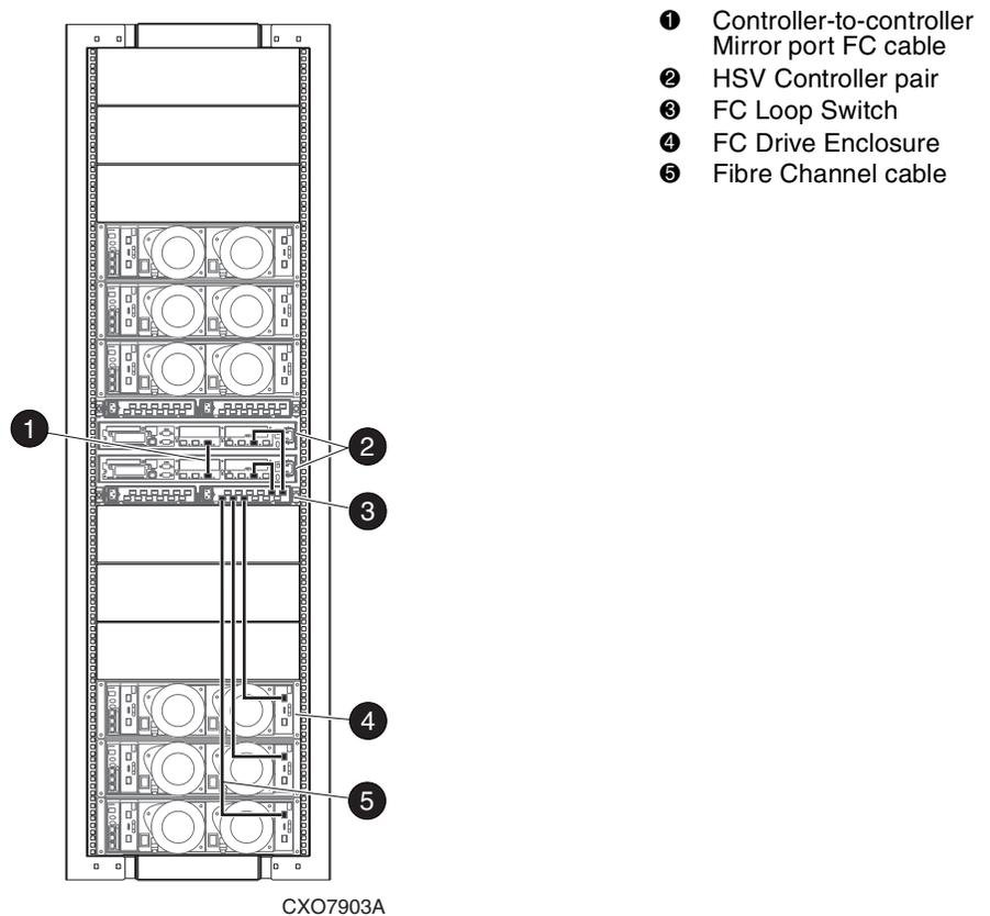
**Figure 2–12: 2C6D configuration—Fibre Channel loop 1A with FC Loop Switch**
