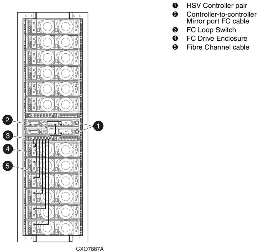
Figure 2–3: 2C12D configuration—Fibre Channel loop 1B with FC Loop Switch
