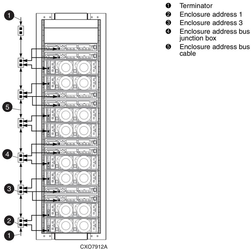
Figure 2–21: 8C8D configuration—enclosure address bus cables
