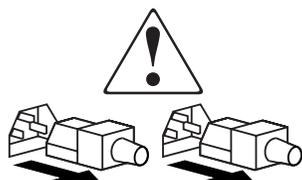
Power supplies or systems marked with these symbols indicate the presence of multiple sources of power.
