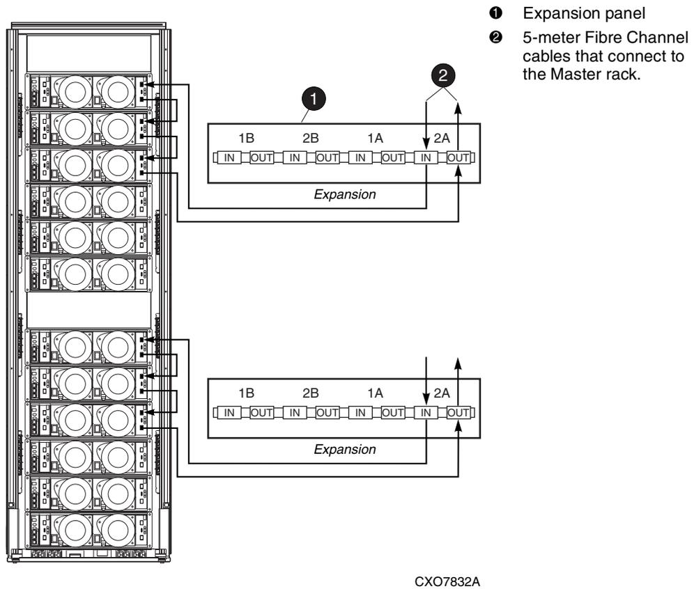
Figure 4–18: 0C6D + 6D configuration—Fibre Channel loop 2A with expansion panels
