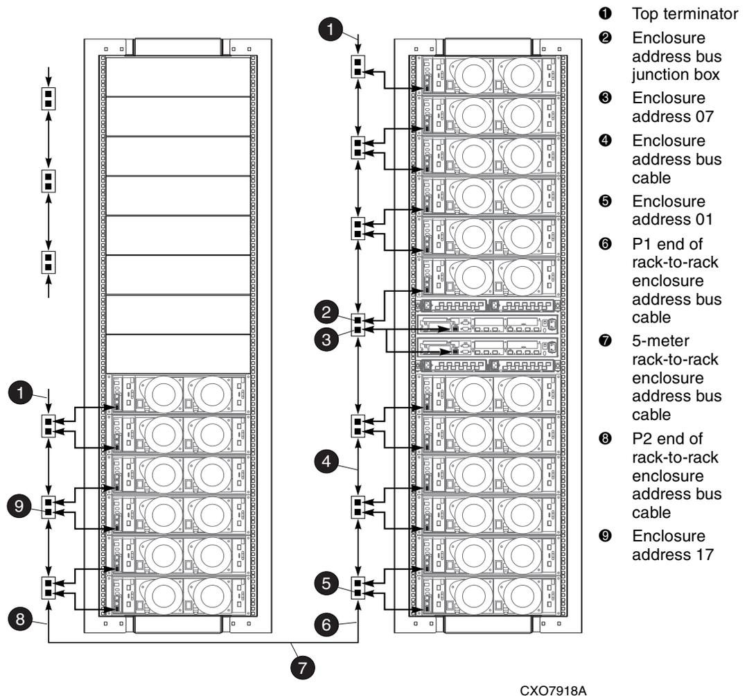
Figure 2–27: 2C12D + 0C6D configuration—enclosure address bus cables
