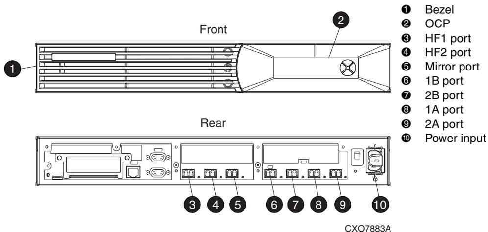
**Figure 1–9: HSV Controller—front and rear views**
