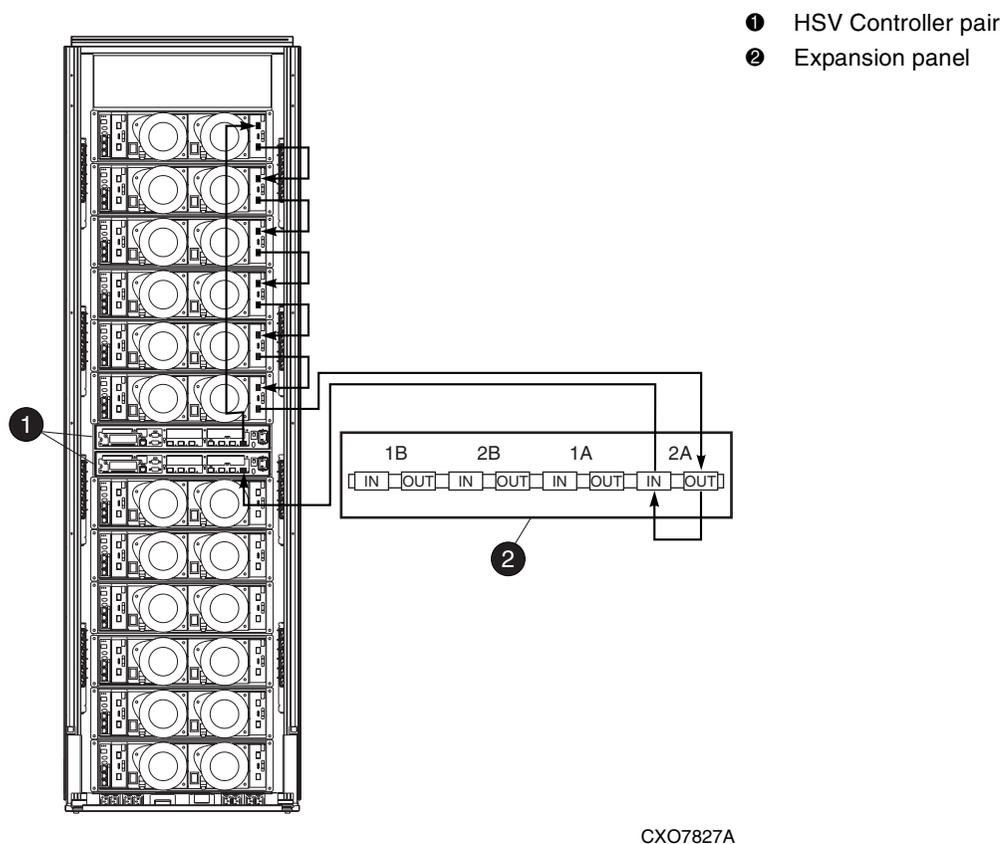
**Figure 4–9: 2C6D + 6D configuration—Fibre Channel loop 2A with expansion panel**
