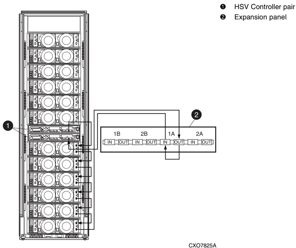
**Figure 4–7: 2C6D + 6D configuration—Fibre Channel loop 1A with expansion panel**
