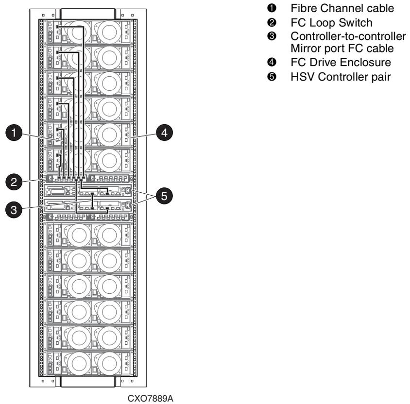
**Figure 4–6: 2C6D + 6D configuration—Fibre Channel loop 2B with FC Loop Switch**
