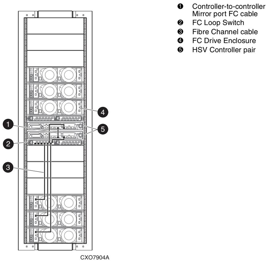
Figure 2–13: 2C6D configuration—Fibre Channel loop 1B with FC Loop Switch
