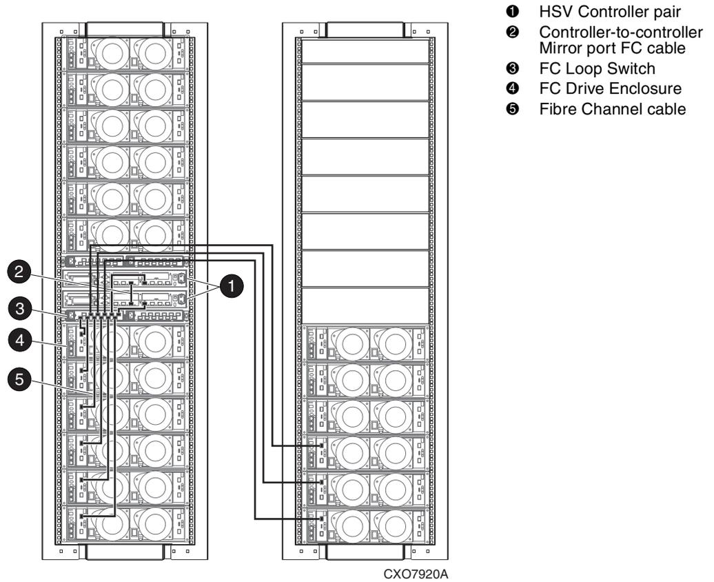
**Figure 2–29: 2C12D + 0C6D configuration—Fibre Channel loop 1B with FC Loop Switch**
