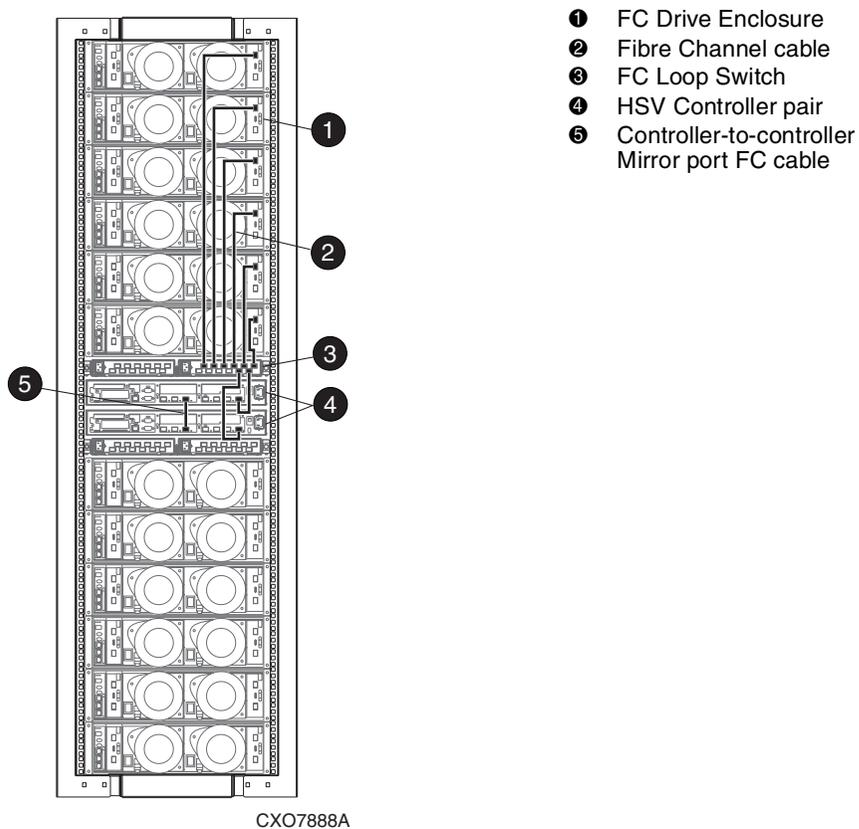
Figure 4–5: 2C6D + 6D configuration—Fibre Channel loop 2A with FC Loop Switch
