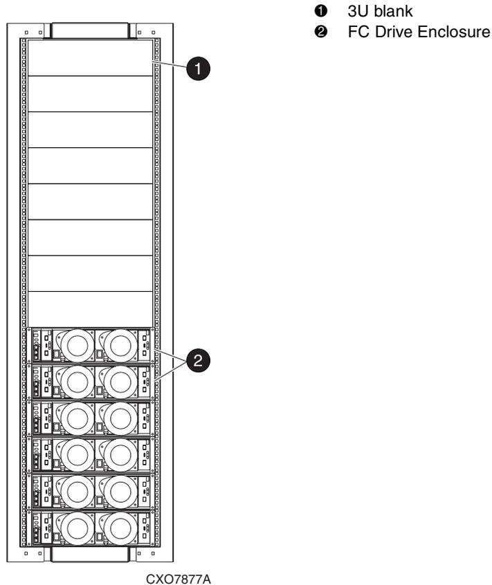
**Figure 1–6: 0C6D configuration—rear view**
