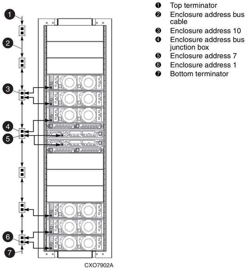
Figure 2–11: 2C6D configuration—enclosure address bus cables
