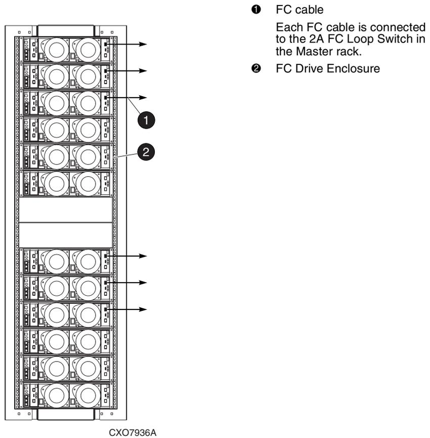
**Figure 4–14: 0C6D + 6D configuration—Fibre Channel loop 2A**
