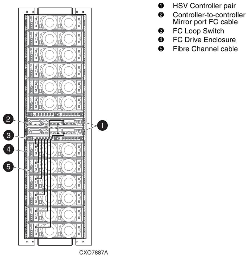
**Figure 4–4: 2C6D + 6D configuration—Fibre Channel loop 1B with FC Loop Switch**
