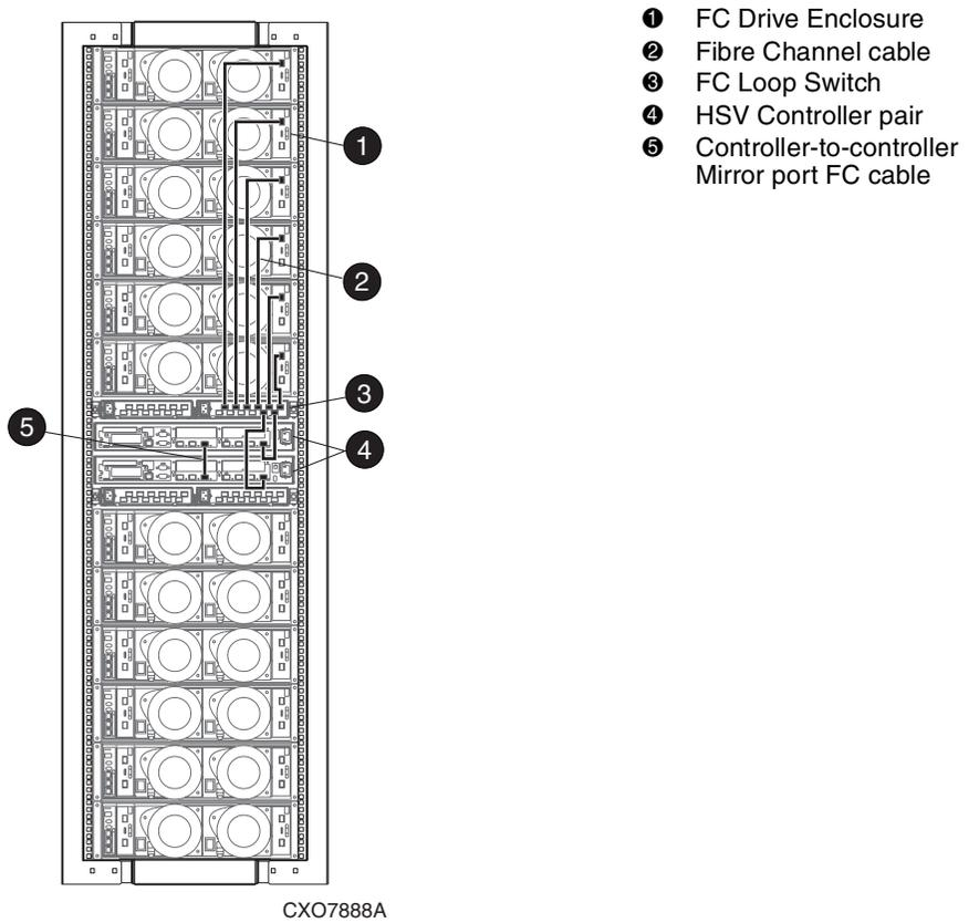
**Figure 2–4: 2C12D configuration—Fibre Channel loop 2A with FC Loop Switch**
