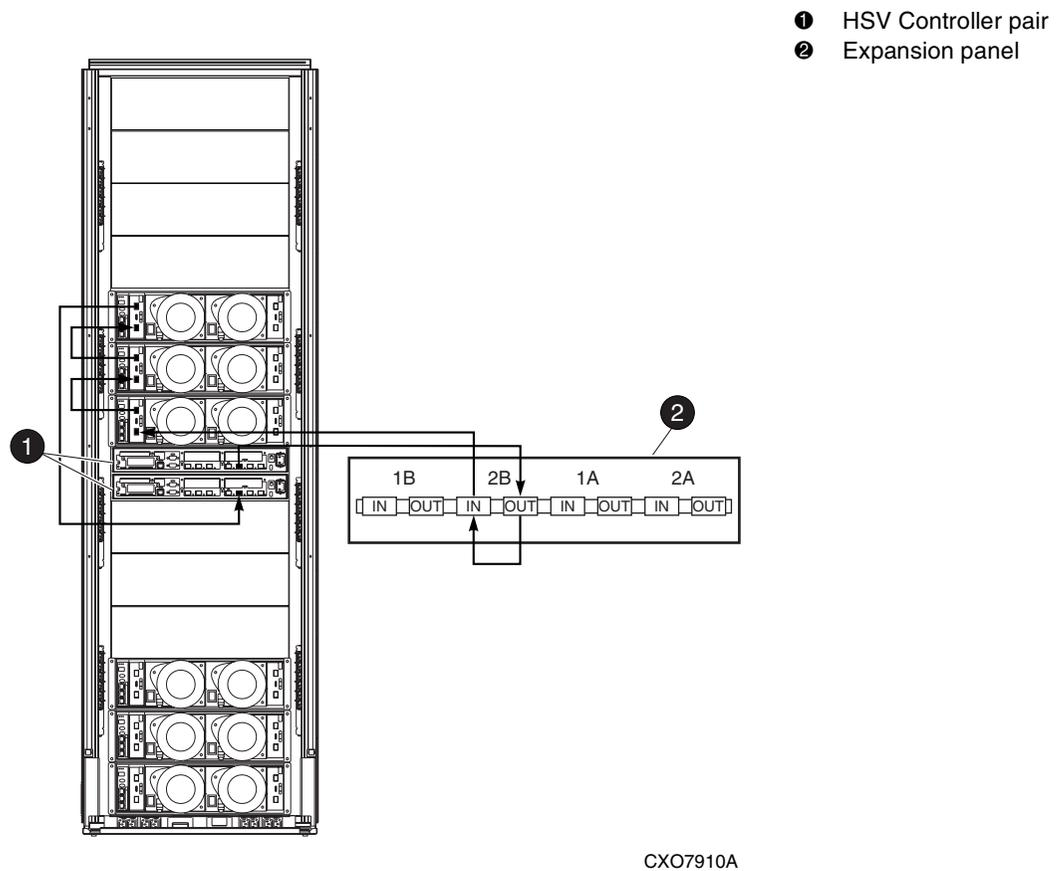
**Figure 2–19: 2C6D configuration—Fibre Channel loop 2B with expansion panel**
