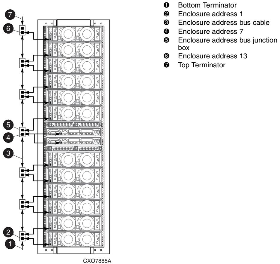
**Figure 2-1: 2C12D configuration—enclosure address bus cables**
