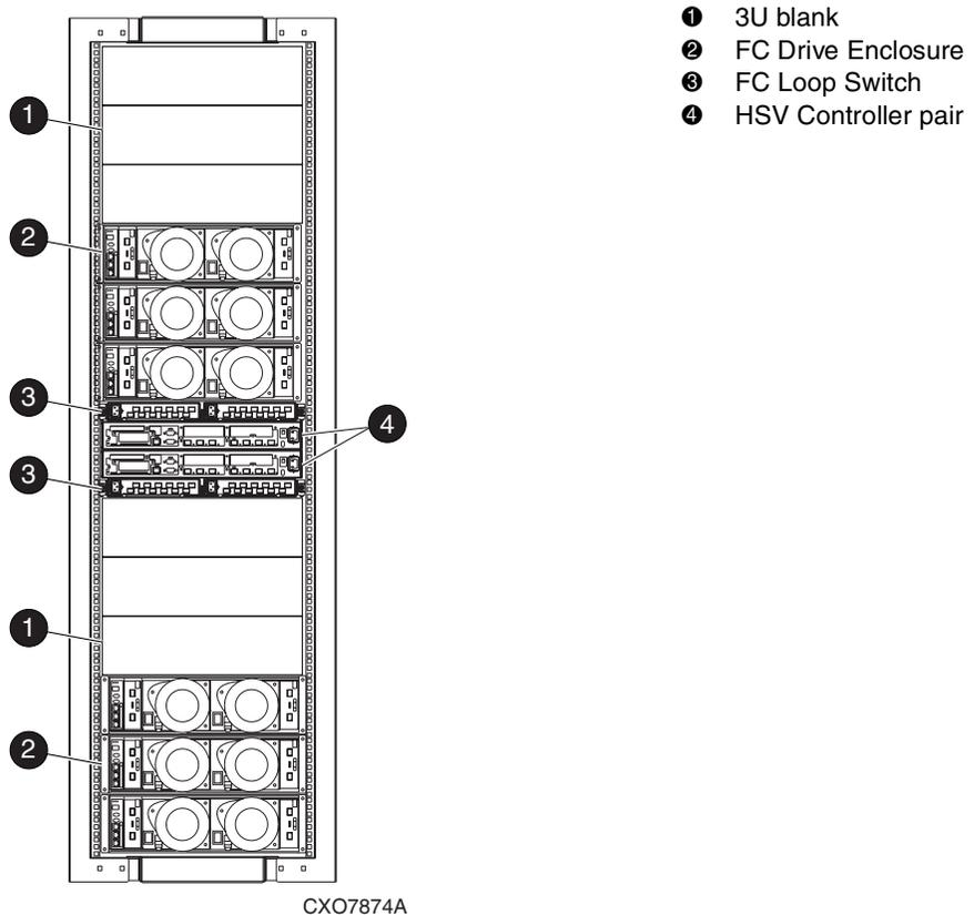
**Figure 1–3: 2C6D configuration—rear view**
