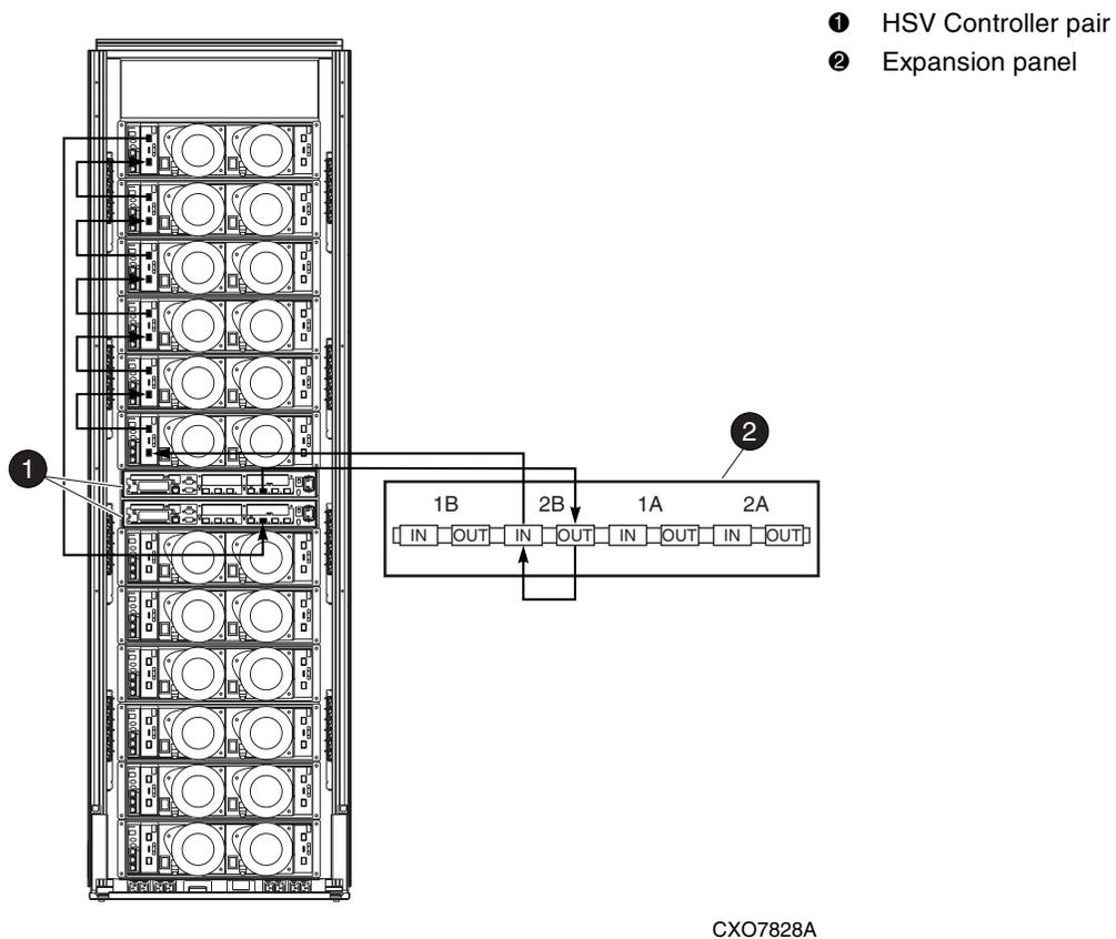
**Figure 4–10: 2C6D + 6D configuration—Fibre Channel loop 2B with expansion panel**
