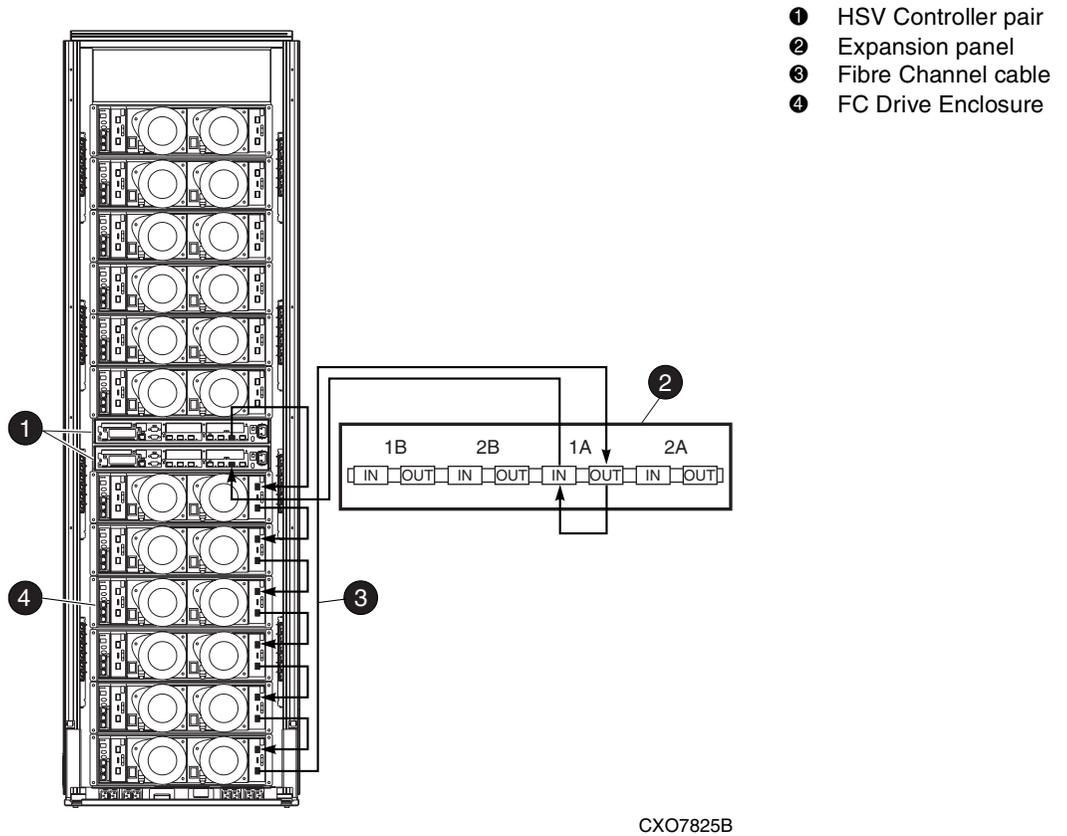
**Figure 2–6: 2C12D configuration—Fibre Channel loop 1A with expansion panel**
