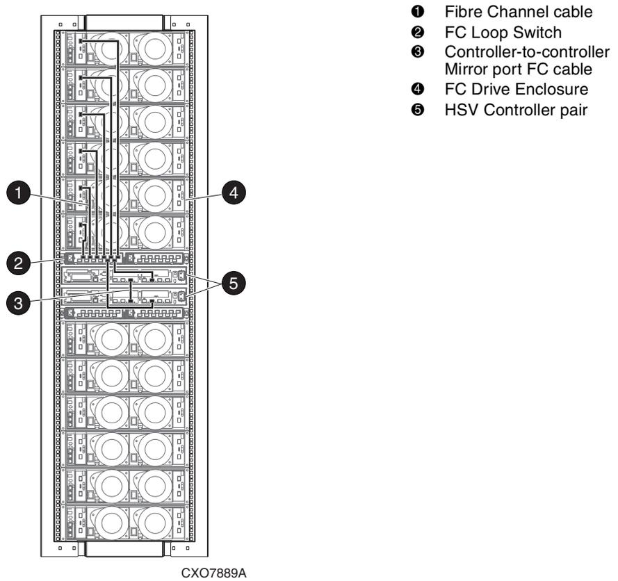
Figure 2–5: 2C12D configuration—Fibre Channel loop 2B with FC Loop Switch
