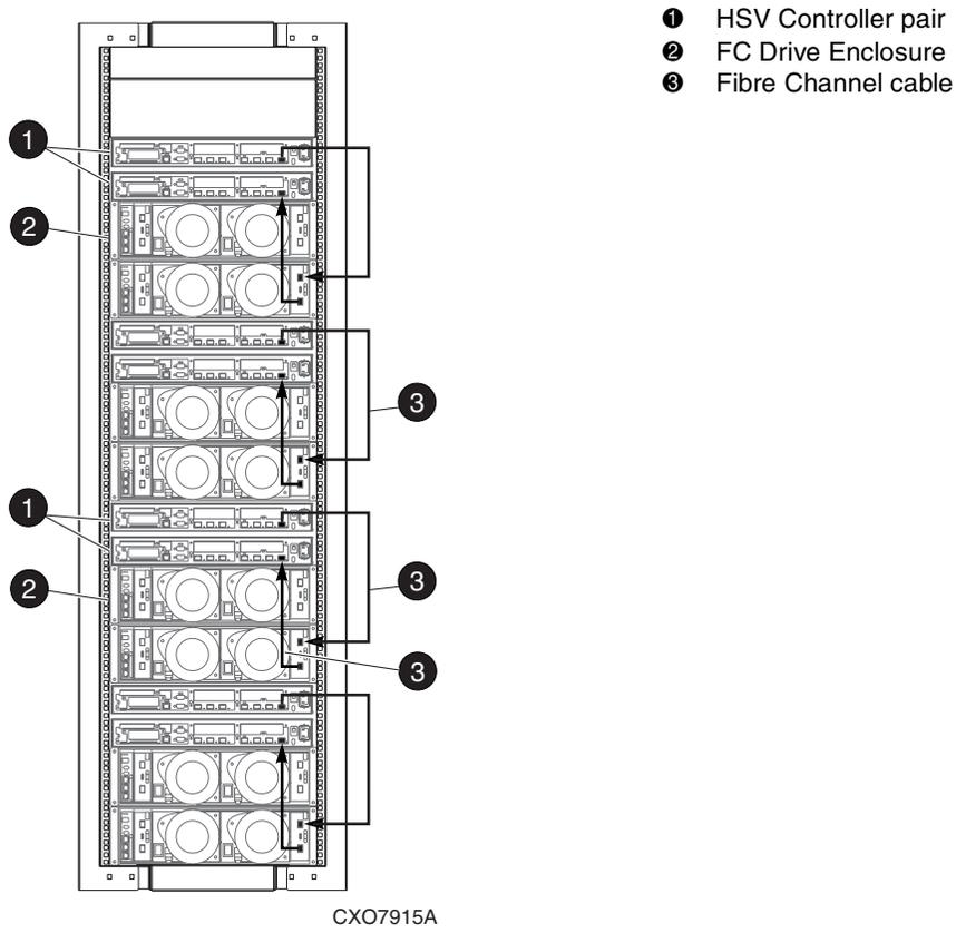
Figure 2–24: 8C8D configuration—Fibre Channel loop 2A
