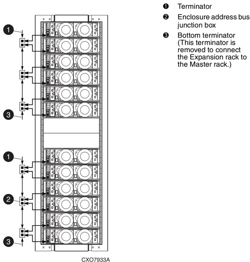
Figure 4–11: 0C6D + 6D configuration—enclosure address bus cables
