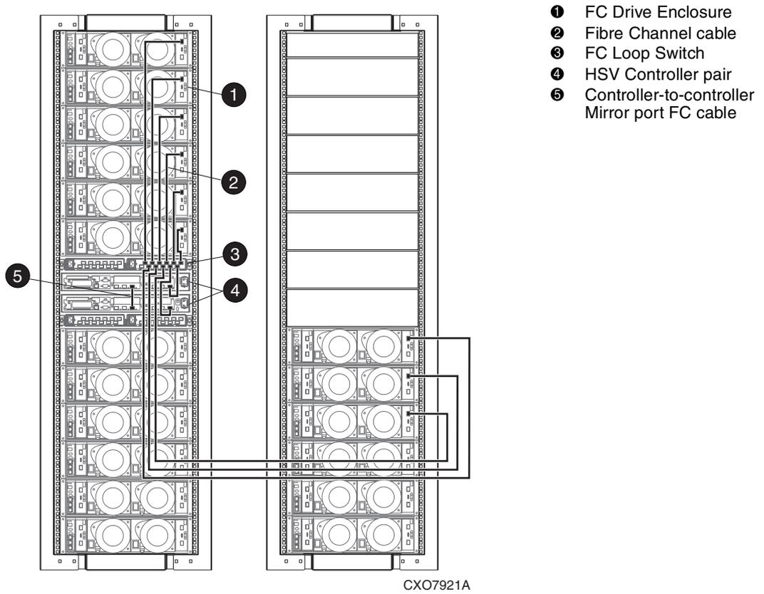
Figure 2–30: 2C12D + 0C6D configuration—Fibre Channel loop 2A with FC Loop Switch
