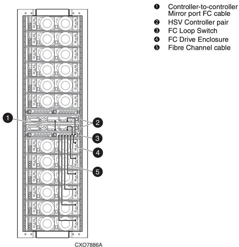
**Figure 4–3: 2C6D + 6D configuration—Fibre Channel loop 1A with FC Loop Switch**
