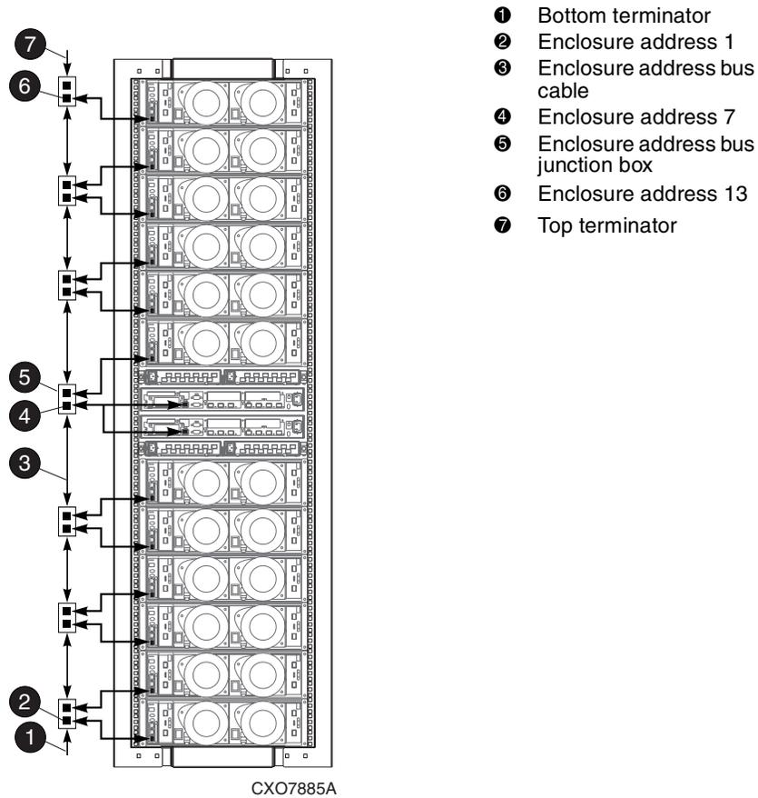
**Figure 4-2: 2C6D + 6D configuration—enclosure address cables**
