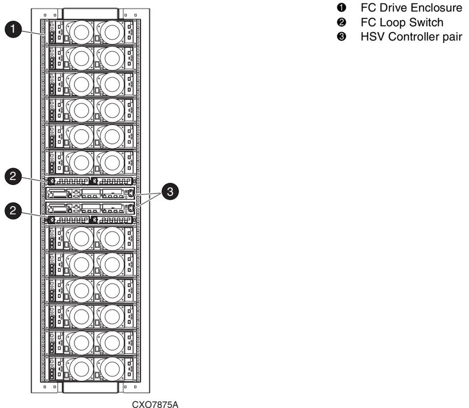
**Figure 1–4: 2C12D configuration—rear view**
