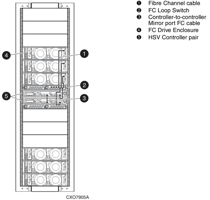
**Figure 2–14: 2C6D configuration—Fibre Channel loop 2A with FC Loop Switch**
