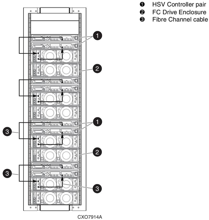
Figure 2–23: 8C8D configuration—Fibre Channel loop 1B
