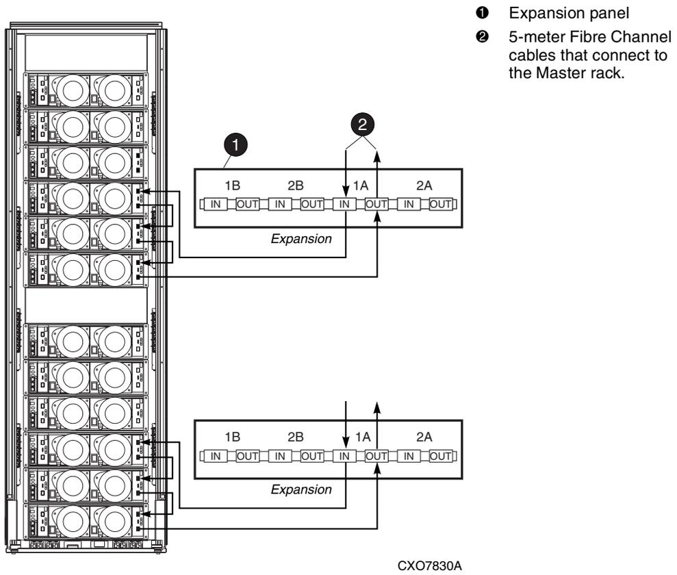
Figure 4–16: 0C6D + 6D configuration—Fibre Channel loop 1A with expansion panels
