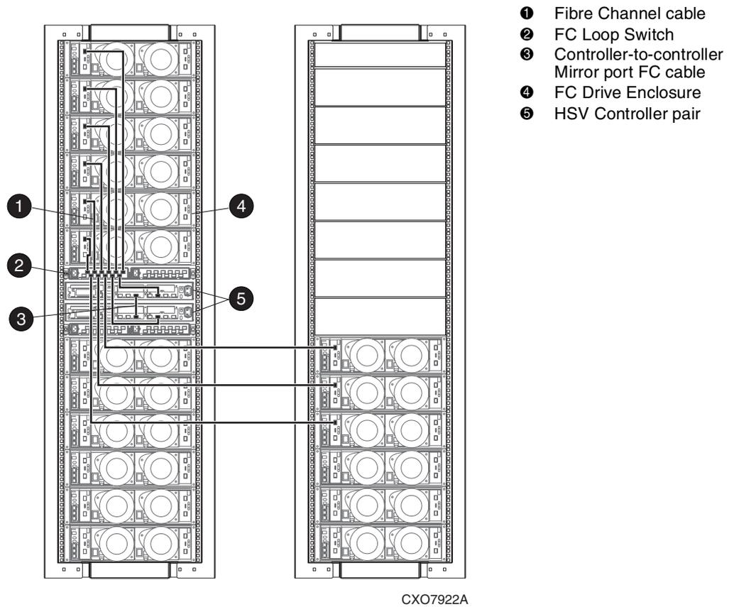
**Figure 2–31: 2C12D + 0C6D configuration—Fibre Channel loop 2B with FC Loop Switch**
