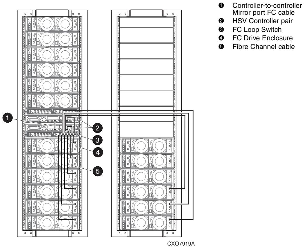
Figure 2–28: 2C12D + 0C6D configuration—Fibre Channel loop 1A with FC Loop Switch
