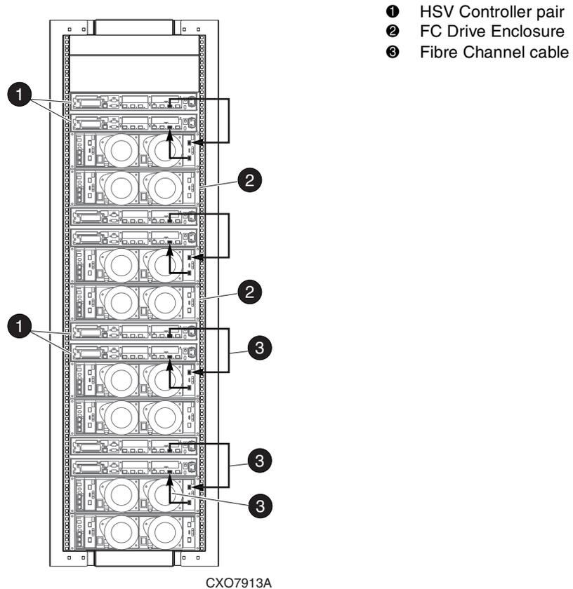
Figure 2–22: 8C8D configuration—Fibre Channel loop 1A
