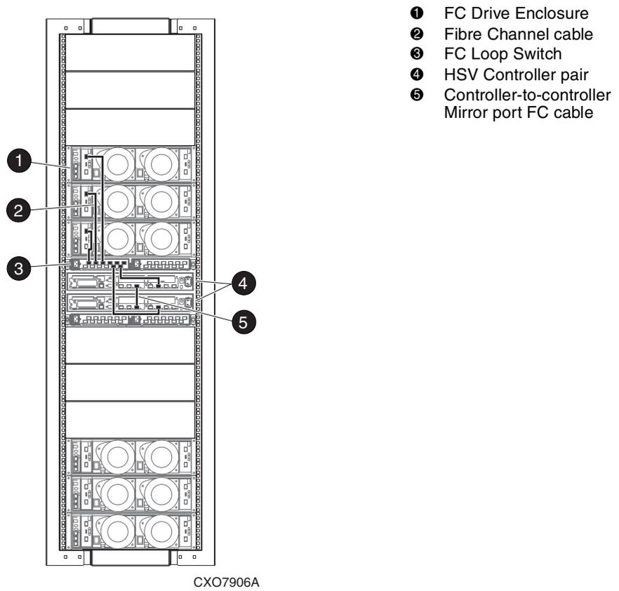
Figure 2–15: 2C6D configuration—Fibre Channel loop 2B with FC Loop Switch
