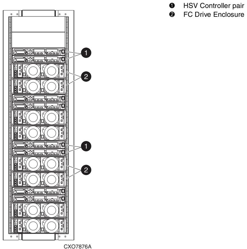
**Figure 1–5: 8C8D configuration—rear view**
