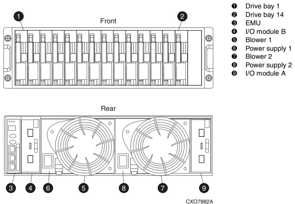
**Figure 1–8: FC Drive Enclosure—front and rear views**
