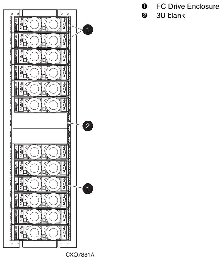
**Figure 1–7: 0C12D configuration—front and rear views**
