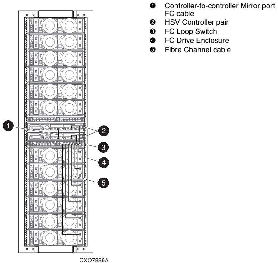
**Figure 2–2: 2C12D configuration—Fibre Channel loop 1A with FC Loop Switch**
