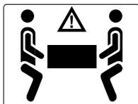
**WARNING:** The weight of the drive enclosure with the elements installed always requires at least two individuals to move. Compaq recommends using a fork lift or a hand truck to move an enclosure in the shipping container.
