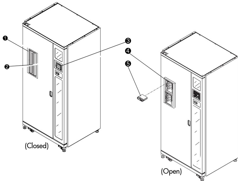
**Figure 20: Load port (ESL9322 shown)**
