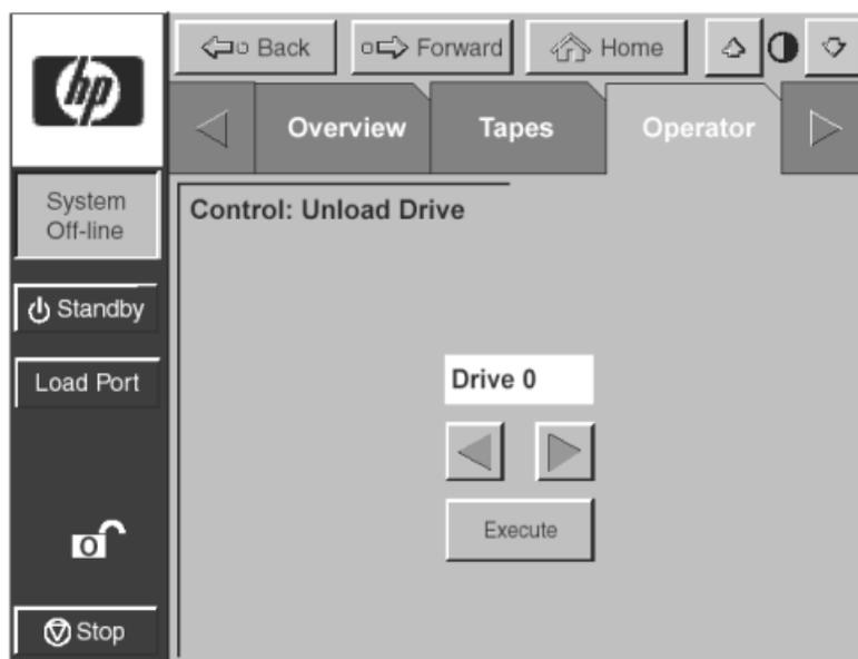
**Figure 35: Control: unload drive screen**
