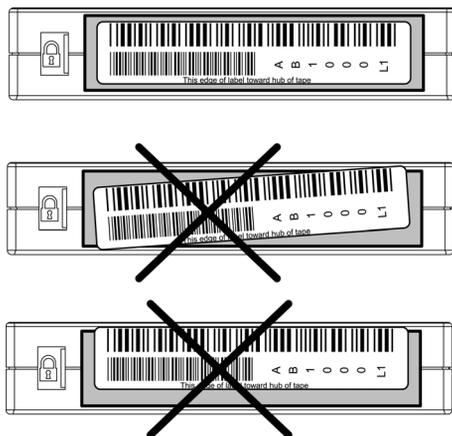
Figure 17: Proper Ultrium bar code label placement
