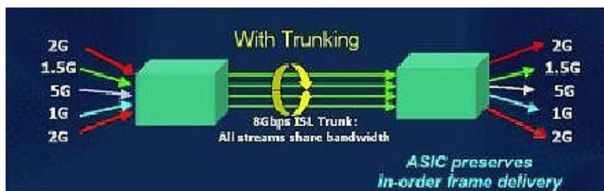
Figure 2: Routing with the ISL Trunking feature
