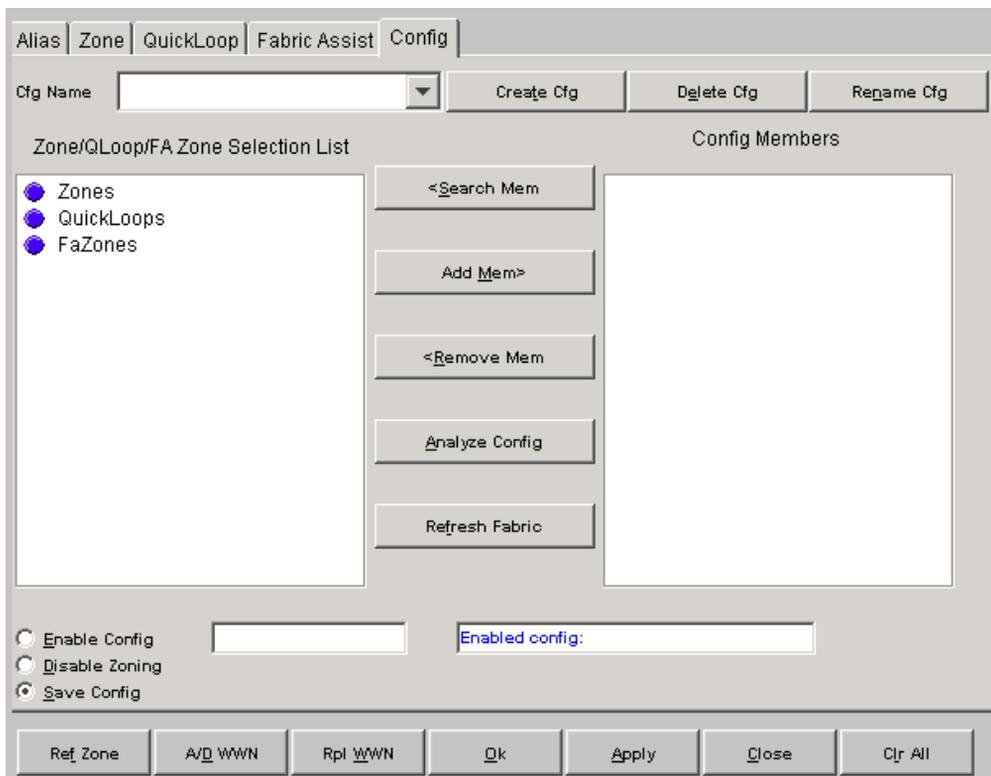
**Figure 3–48: Config Tab of the Mixed Level Zoning menu**
