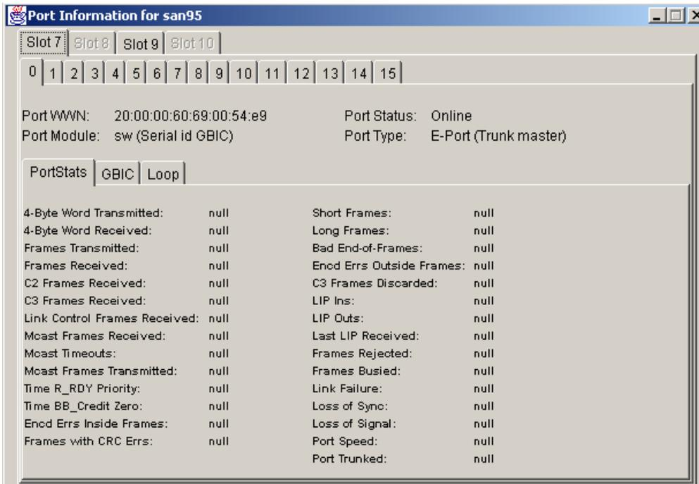
**Figure 5–6: The PortStats tab in the Port Information view**
