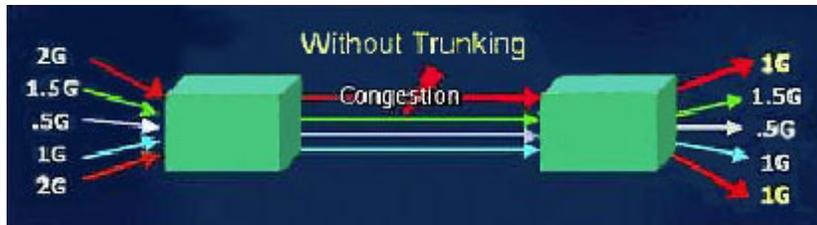
Figure 1–1: Routing without the ISL Trunking feature
