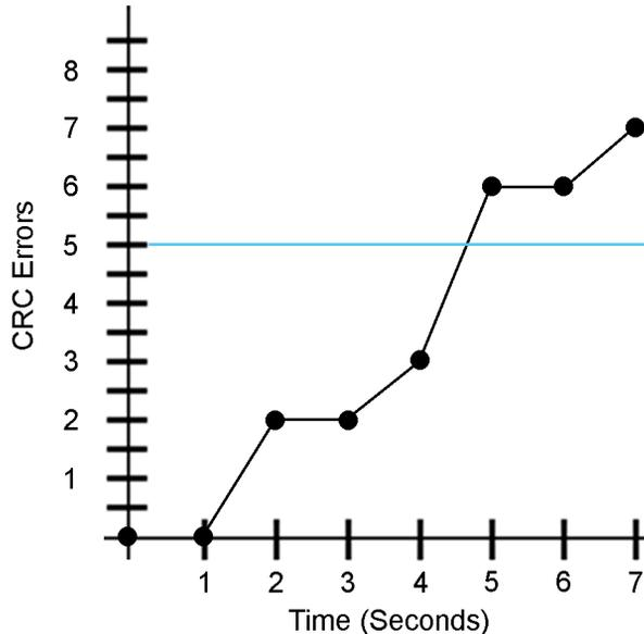
Figure 1–2: Rising/Falling Threshold
