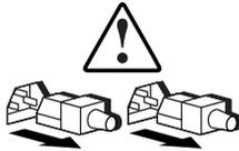
Power Supplies or Systems marked with these symbols indicate the equipment is supplied by multiple sources of power.
