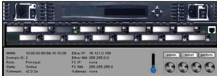
Figure 3-4. General Switch View—Compaq StorageWorks SAN Switch 16
