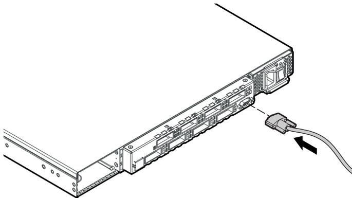
Figure 2-4. Connecting the serial cable
