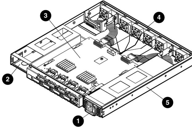
Figure 6-1. Switch components
