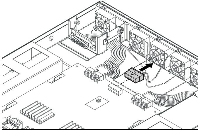
Figure 6-6. Disconnecting the wiring harness
