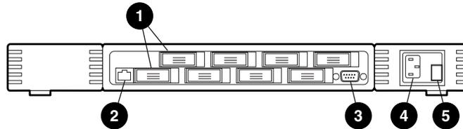
Figure 1-1. Fibre Channel SAN Switch 8 front panel
