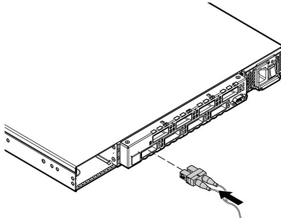
Figure 2-2. Connecting a cable to a GBIC module in a Fibre Channel port
