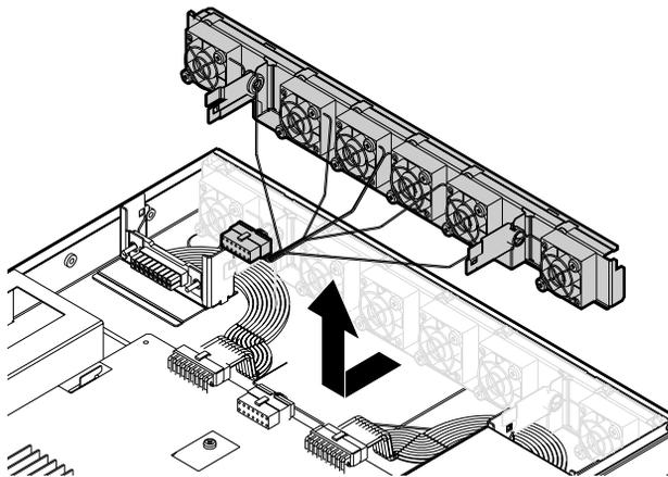
Figure 6-7. Removing the fan assembly
