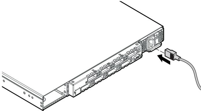
Figure 2-3. Connecting the power cord
