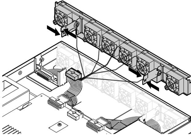
Figure 6-8. Releasing the tabs on the fan assembly
