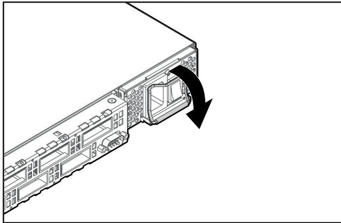
Figure 6-2. Metal handle on the power supply unit
