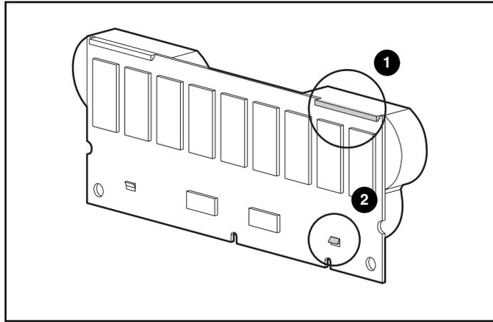
**Figure 10: Securing the battery pack**
