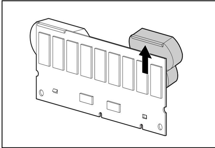
**Figure 8: Removing the battery pack**
