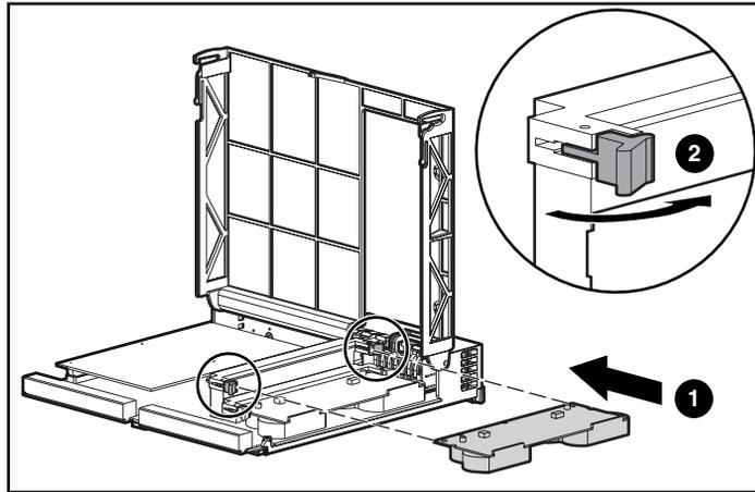
**Figure 4: Installing the cache module**
