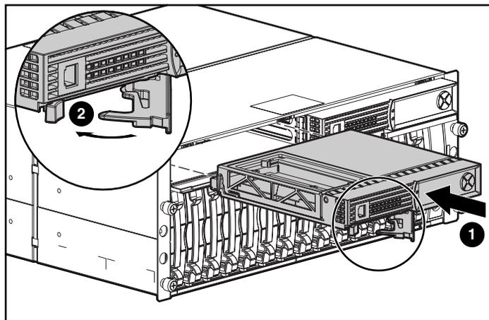
**Figure 13: Installing the replacement controller**
