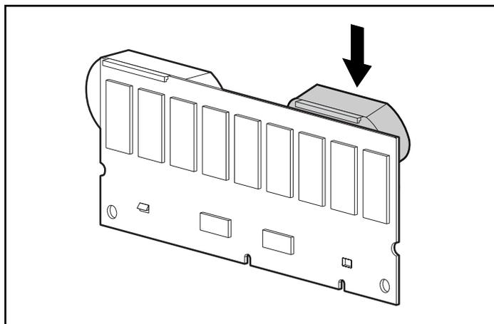
**Figure 9: Installing the battery pack**
