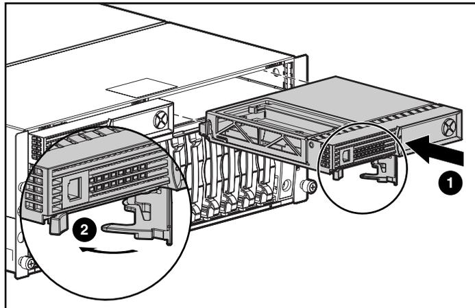
**Figure 5: Installing the controller**
