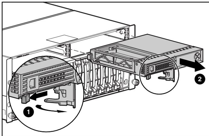
**Figure 12: Removing the MSA1000 Controller**
