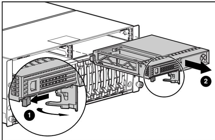
**Figure 2: Removing the controller**
