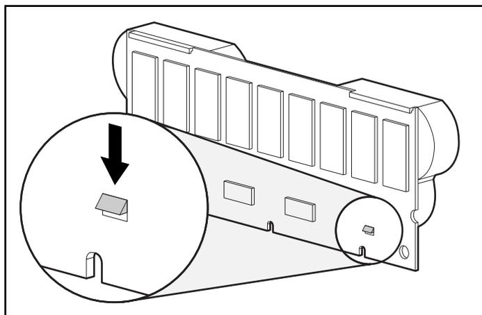
**Figure 6: Bottom clip on battery pack**
