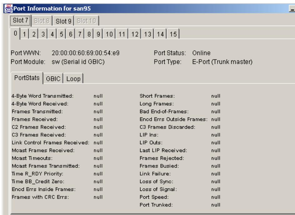
**Figure 135: The PortStats tab in the Port Information view**
