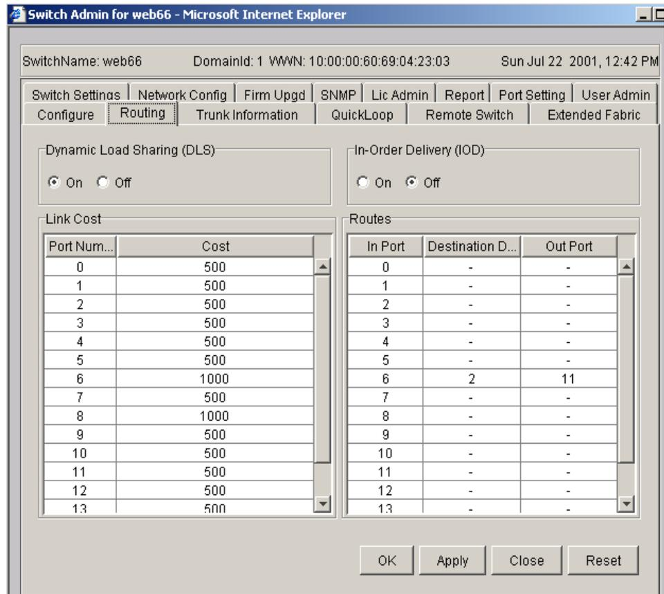
**Figure 113: Routing tab**
