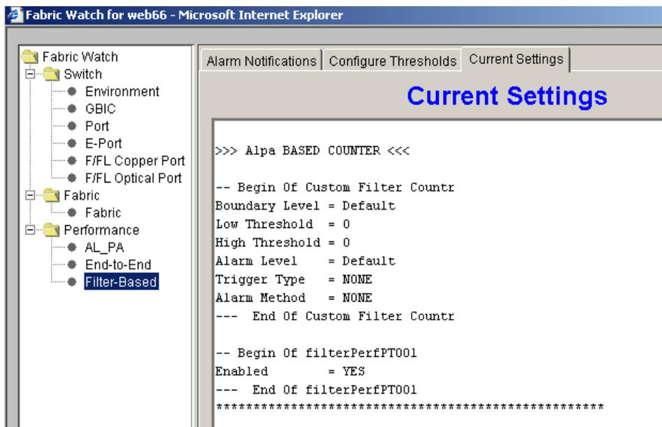
Figure 63: Current Settings tab in the Fabric Watch view
