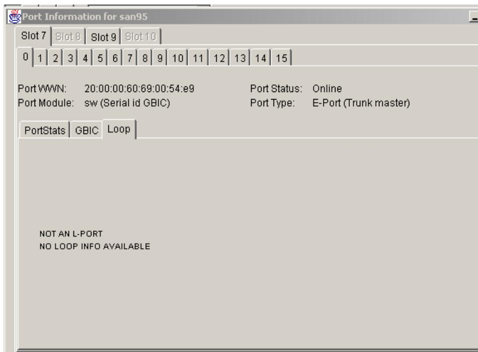
**Figure 137: The Loop tab in the Port Information view**
