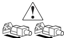
Power supplies or systems marked with these symbols indicate the presence of multiple sources of power.
