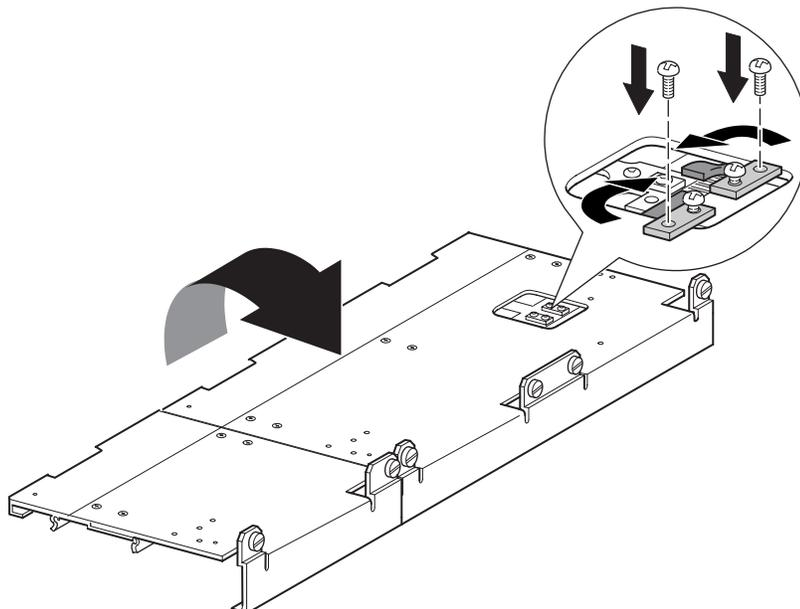
**Figure 2–19: Timing belt at the belt block**
