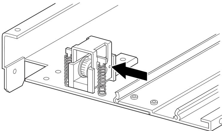
**Figure 2–16: Tensioner ramp/idler pulley zero point**
