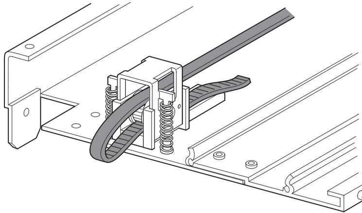
**Figure 2–17: Installing the timing belt on the extension**
