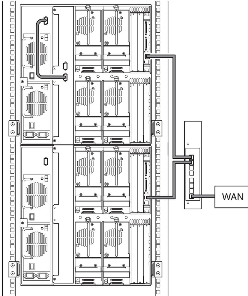
**Figure 2–21: MSL5052 multi-unit library configuration (single master and slave)**
