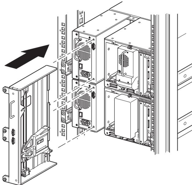
**Figure 2–6: Installing the PTM base unit**
