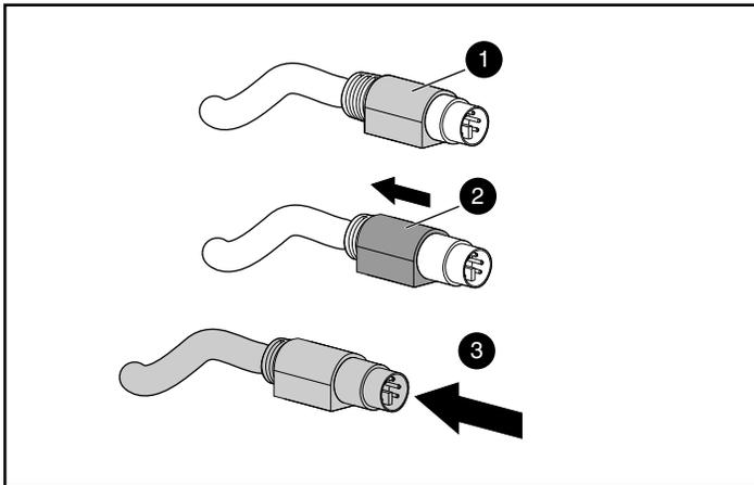
To insert the cable, simply plug it into the appropriate connector. The locking mechanism automatically locks the cable in place.
