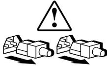
Power Supplies or Systems marked with these symbols indicate the equipment is supplied by multiple sources of power.
