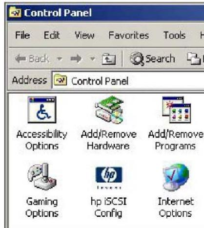
Open the *hp iSCSI Config* configuration screen and add the IP addresses of the newly created SCSI Router Instances from each SR2122-2 Node A and Node B, 33.33.33.103 and 33.33.33.104 respectively
