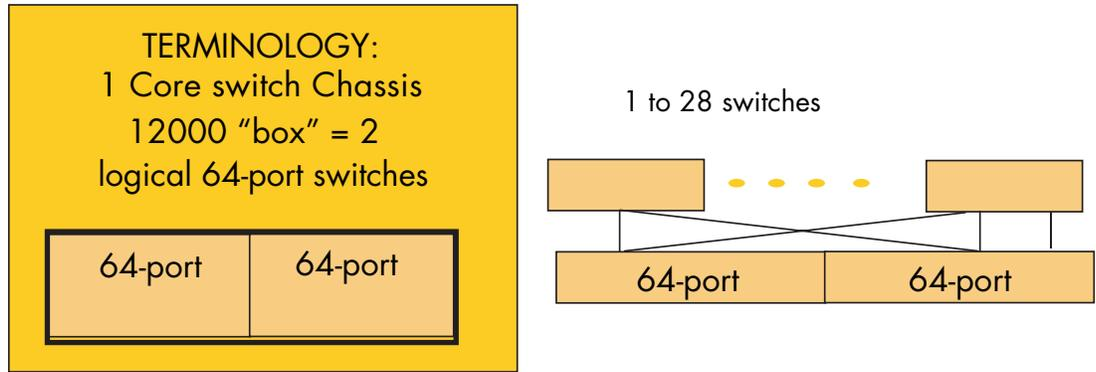
Figure 22: Core Switch definition and SAN fabric with up to 16 switches
