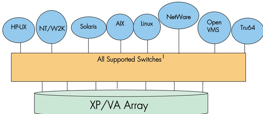
**Figure 31: XP/VA with multiple OS's on a shared SAN fabric<sup>1</sup>**
