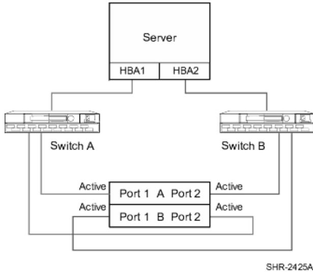
**Figure 38: Cross-Cable High Availability NSPOF Configuration**
