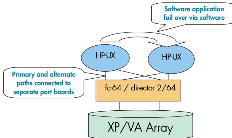
Figure 30: Software application fail-over
