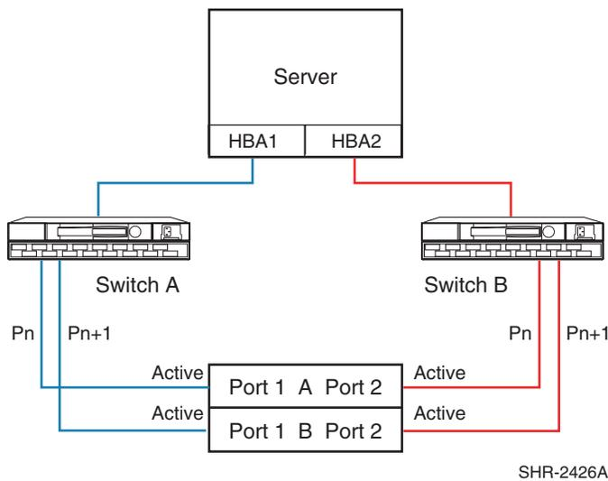
**Figure 39: Straight-Cable High Availability NSPOF Configuration**
