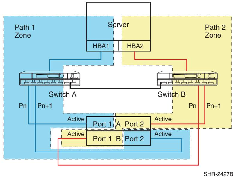
**Figure 40: Cross-Cable High Availability Single Fabric Zoned Configuration**
