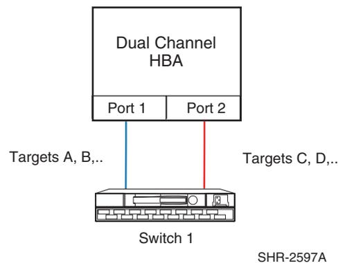
**Figure 42: Single PCI Slot with Dual Channel HBA and One Switch**
