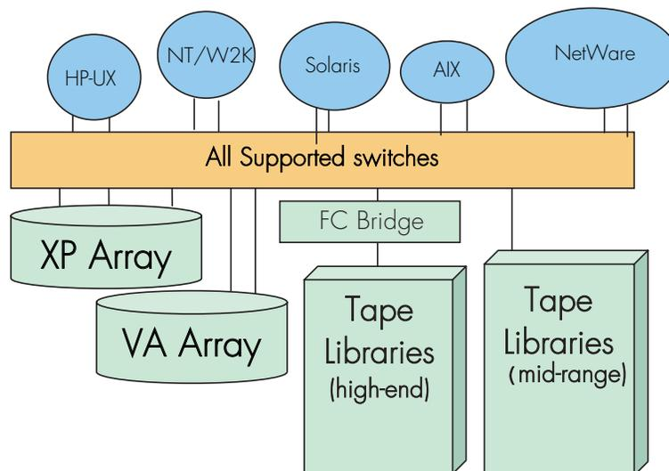
Figure 32: XP/VA with multiple OS's and tapes on a shared SAN fabric, fabric only<sup>1</sup>
