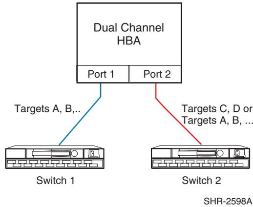
**Figure 43: Single PCI Slot with Dual Channel HBA and Two Switches**
