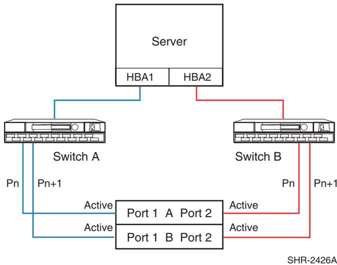
**Figure 38: Straight-Cable High Availability NSPOF Configuration**
