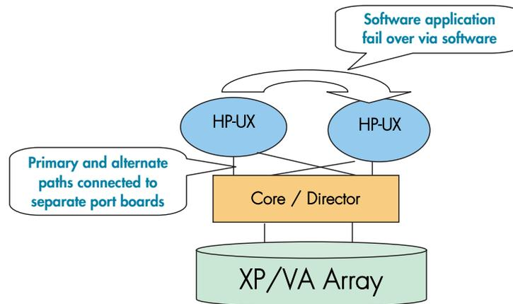
**Figure 29: Software application fail-over**
