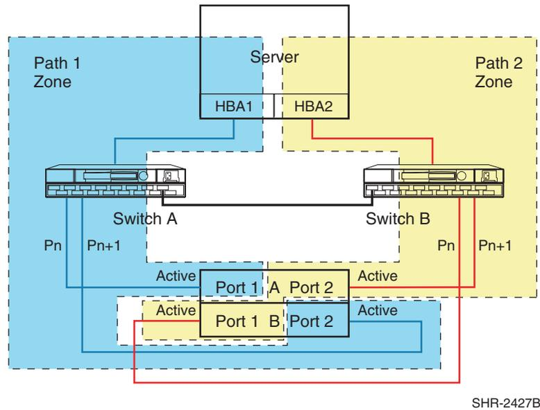
**Figure 39: Cross-Cable High Availability Single Fabric Zoned Configuration**
