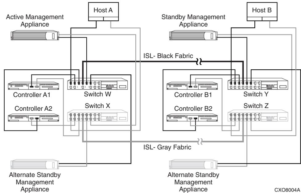
**Figure 48: Continuous Access EVA basic configuration**
