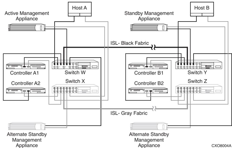
**Figure 44: Continuous Access EVA basic configuration**
