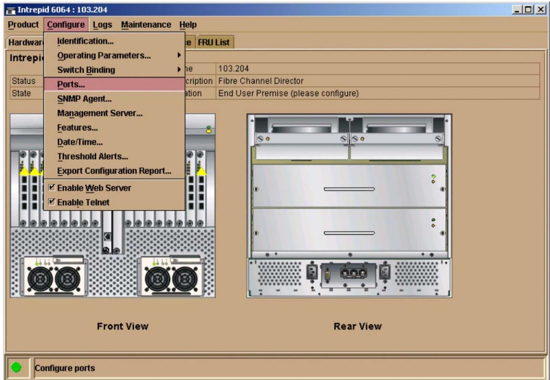
Figure 32: HAFM: Select Configure > Ports
