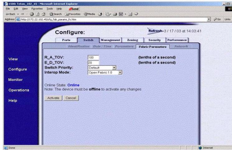
Figure 26: EWS: Selecting Fabric Parameters Tab
