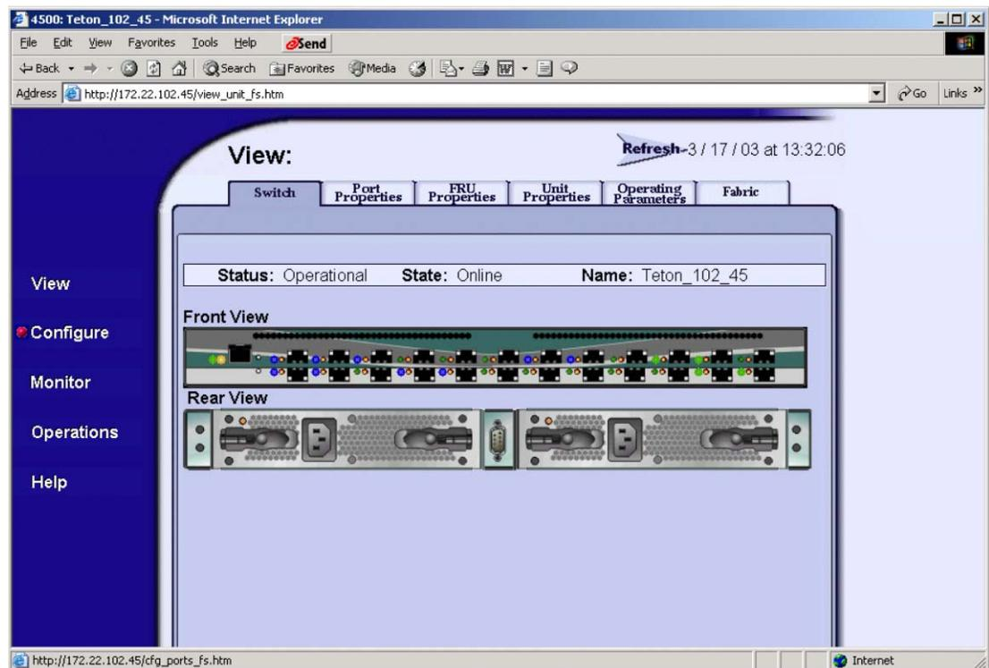
Next, you can select the port speed for each port. Remember, any ports connecting to a SAN Switch 2/8 or 2/16 must be set to 2 Gb/sec. See ports 0-3 as an example.
