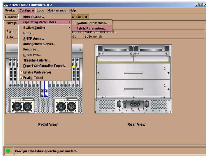
Figure 19: HAFM: Selecting Configure Operating Parameters for Fabric
