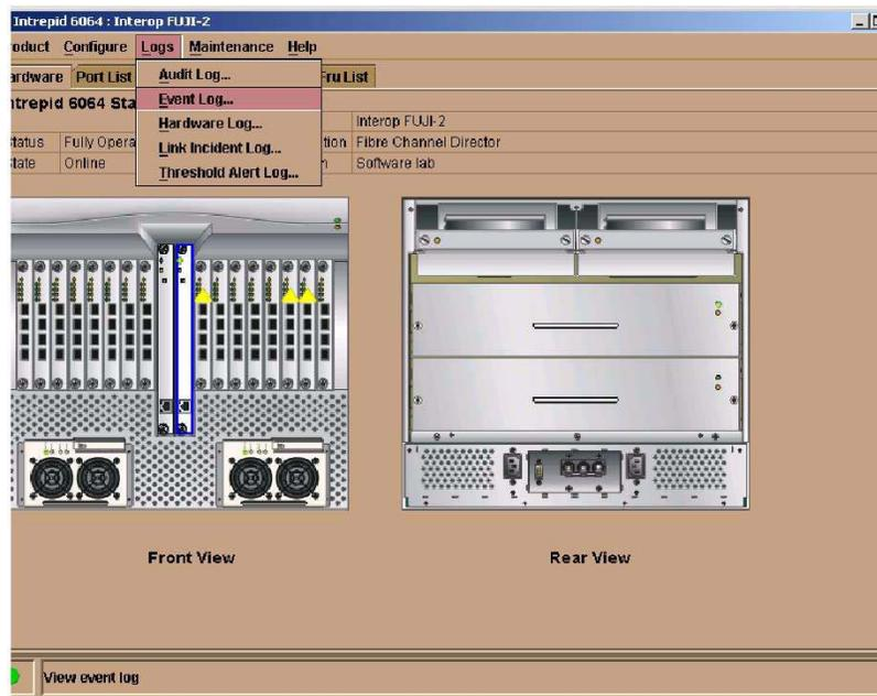
Figure 42: HAFM: Selecting View Event Log for Segmentation Errors
