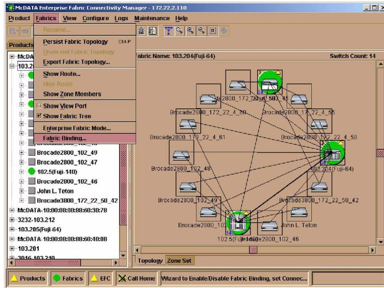
Figure 36: HAFM: Selecting Fabric Binding and Enterprise Fabric Mode
