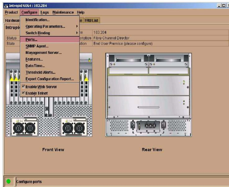
Figure 27: HAFM: Selecting Configure Ports
