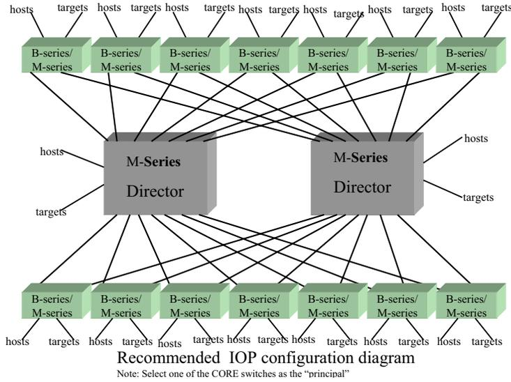
**Figure 9: Core/Edge SAN Configuration with M-Series Director at the Core**
