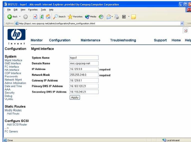
**Figure 32: Valid SR2122 Management Port TCP/IP Configuration**
