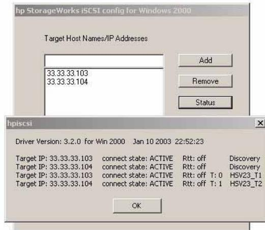
**Figure 28: Checking that SR2122 Targets are Active**
