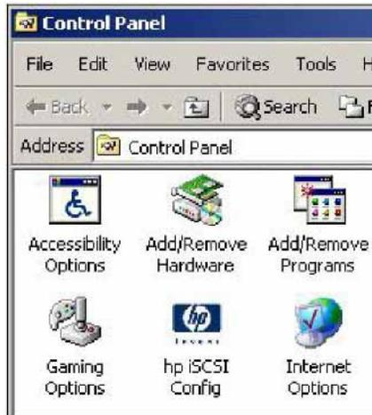
Open the *hp iSCSI Config* configuration screen and add the IP addresses of the newly created SCSI Router Instances from each SR2122 Node A and Node B, 33.33.33.103 and 33.33.33.104 respectively
