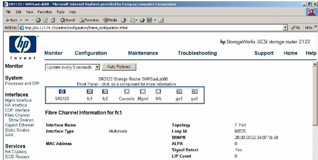
Figure 2: GUI Display of the FC port WWPN
