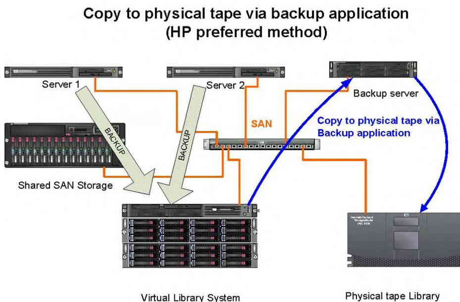
HP strongly recommends the use of the backup application to migrate data from the HP VLS6000 system to physical tape because using the backup application means all the media (virtual and physical) is tracked in the backup application catalog. This ensures reliable, robust data recovery.
