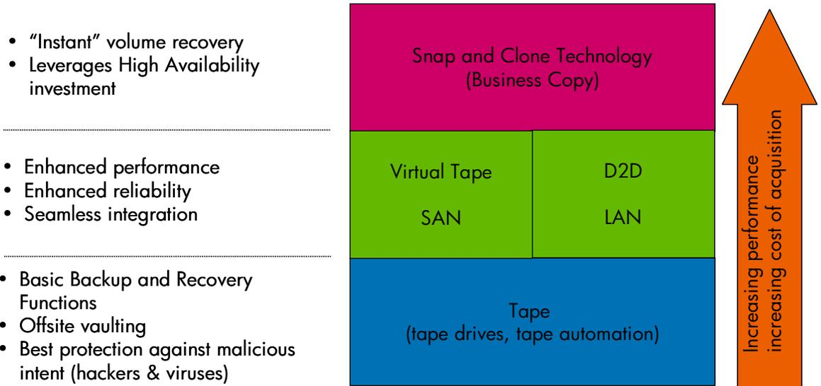
Physical tape will always be the foundation of a robust data protection strategy offering low cost/GB storage and off-site vaulting capabilities. However, in many cases an increase in backup performance can be achieved by using disk-assisted backup techniques<sup>1</sup>.
