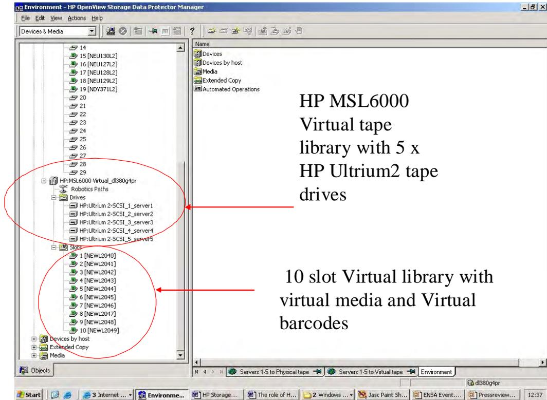
Viewing the virtual tape library (created with five Ultrium 2 drives, 10 slots and each slot loaded with 50-GB media), you can see it appears in exactly the same format as the physical library. The media in the slots each contains a barcode for tracking that was created within the barcode template for the virtual tape library (see Appendix C).
