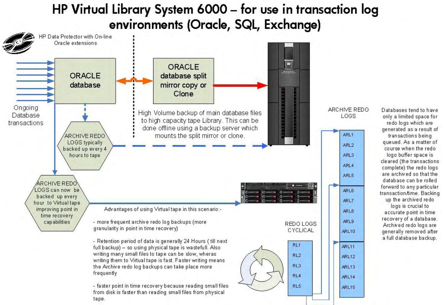
Figure 11 illustrates a familiar concept in database-driven applications—that of redo logs (or, transaction logs). These logs are critical in being able to recover a database to a given point in time (PIT). The logs are only needed in between full backups to roll the database forward or back to a given PIT, and backing them up to tape can be quite a slow process. The benefits of using virtual tape include:
