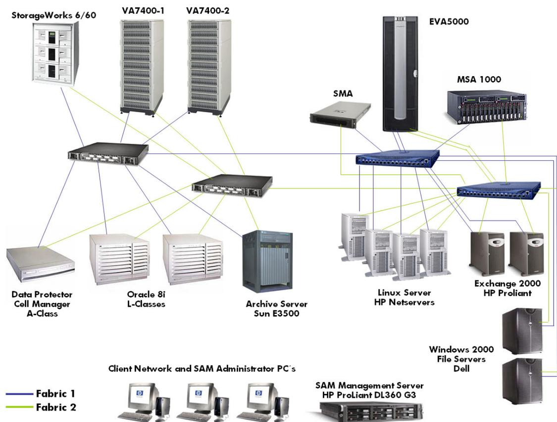
As indicated in Figure 2, the SAN infrastructure provides two redundant SANs for maximum uptime.
