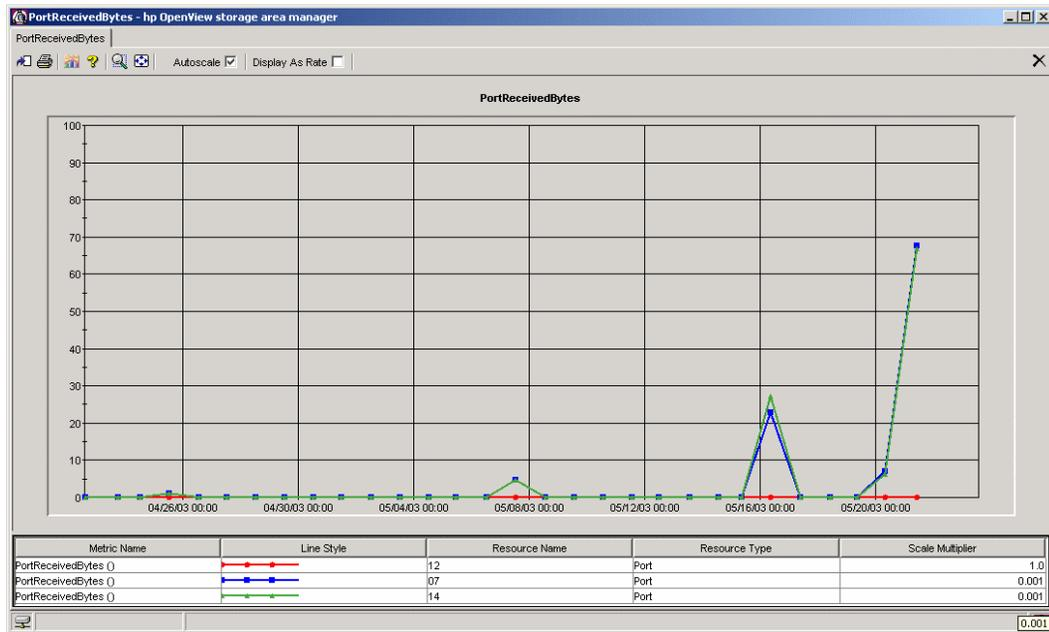
**Figure 5.** Text-based query across all Fibre Channel switches in the domain, using a characteristic throughput metric—Device Received Bytes—as a measure to compare all four switches and identify potential hot spots.
