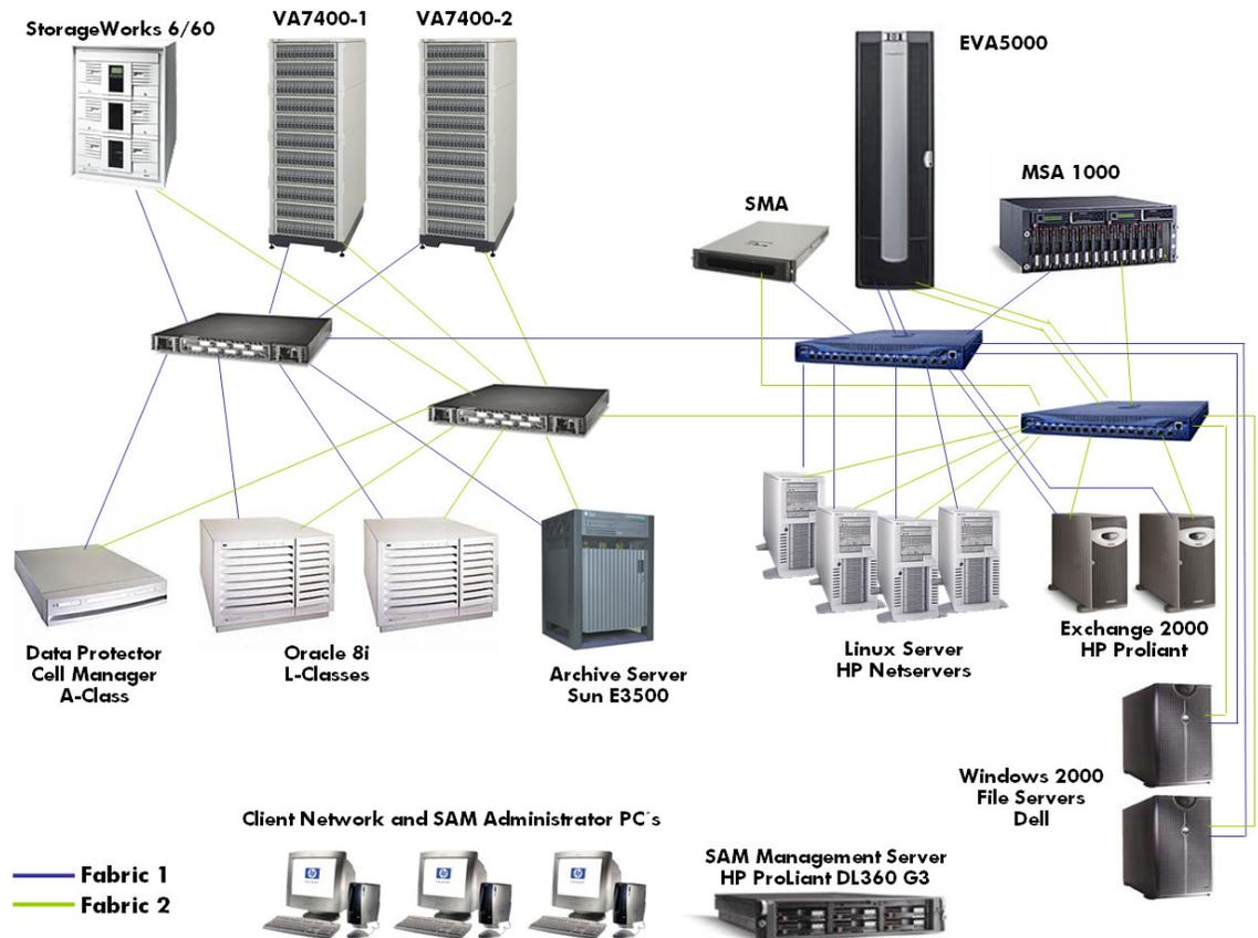
As indicated in Figure 2, the SAN infrastructure provides two redundant SANs for maximum uptime and performance.
