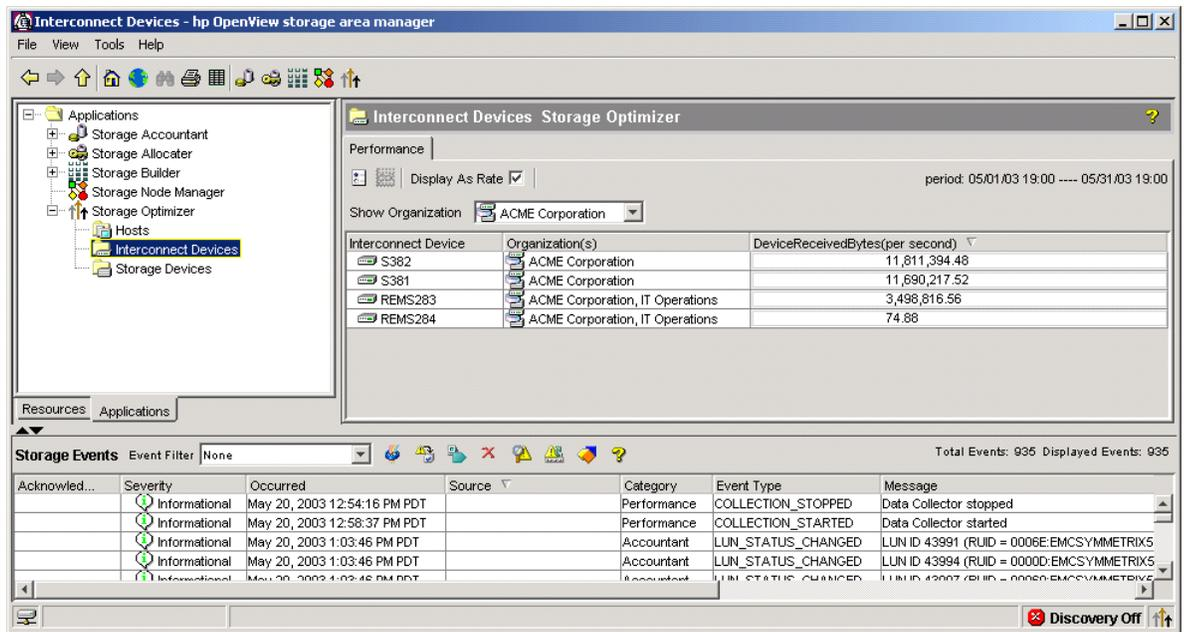
**Figure 6.** Storage Optimizer detail screen. The upper right part of the screen shows Fibre Channel switch port performance counters for Port Total Errors. This metric is used to identify errors on a Fibre Channel connection. An excessive number might indicate cabling or Gigabit Interface Connector (GBIC) problems.
