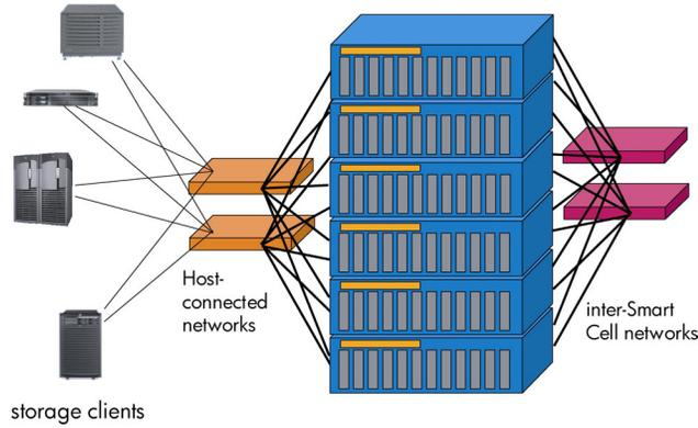
**Figure 4.** Conventional array controller and HP StorageWorks grid
