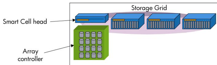
HP StorageWorks RISS, a powerful ILM solution, now offers a first look at an HP StorageWorks grid solution (Figure 8). In the HP RISS, Smart Cells—shown as cubes in the figure—consist of several disk drives that are controlled by an intelligent module. The module incorporates data placement, index, search, and retrieval services as well as the intelligence and connectivity to enable all modules to be federated into a single managed entity—an HP StorageWorks grid.
