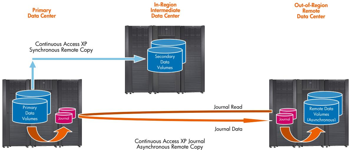
3DC multi-target provides independent replication paths to two recovery sites, and delivers the best protection against a wide range of potential outages at any site.
