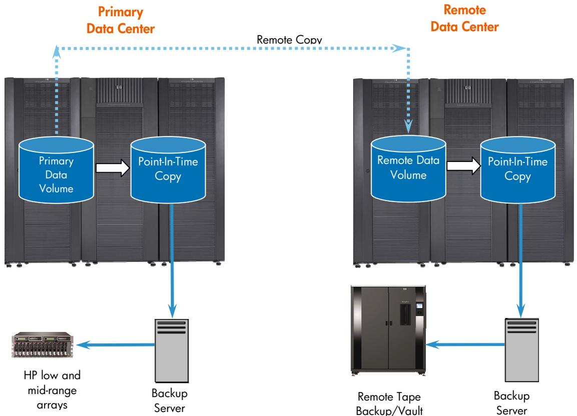
XP12000 Disk Array provides remote replication and point-in-time copy capabilities—including HP StorageWorks Continuous Access XP Journal and HP StorageWorks Business Copy XP software—that enable cost-effective backup to tape or to disk.
