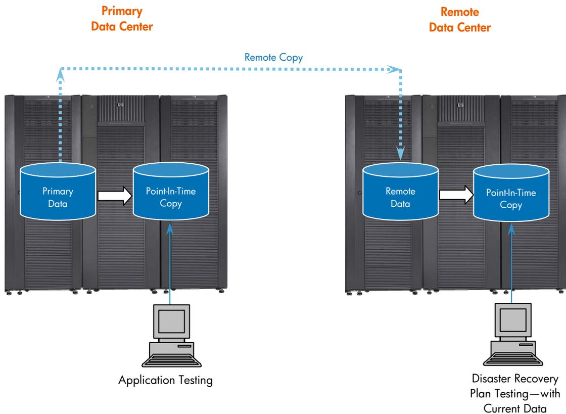
Enterprises use solutions such as Continuous Access XP, Continuous Access XP Extension, or Continuous Access XP Journal software to create a remote copy for disaster recovery. Business Copy XP software provides point-in-time copies for testing.
