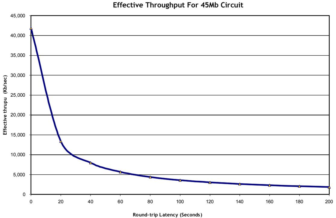
Figure 1 illustrates this problem from a very practical perspective. This graph shows the performance of a TCP data transfer when the network is experiencing a low degree of network loss (less than 1/10 of 1 percent) for increasing amounts of latency. The curve illustrates the performance impact of the protocol window at higher bandwidths.
