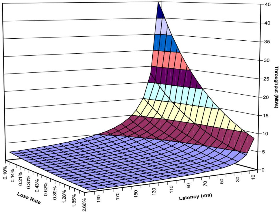
To summarize, Figure 2 graphs a surface of modeled TCP throughput over a 45 Mbps T3 link, as a function of both RTT and loss rates. This graph shows that both loss and latency impact performance. While latency has the more dramatic impact, they combine to severely impact performance. In environments with relatively low loss rates and normal WAN latencies, throughput can be dramatically limited.
