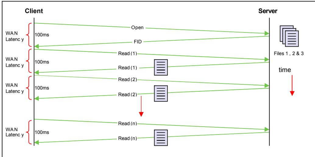
Figure 5 shows how latency affects the performance of client server interactions. In this example, each block is read serially as each round trip is completed. Latency does not have a big effect on performance when the RTT is below 1 ms, like on a LAN. However, when latency is high, taking many round trips degrades performance markedly. In Figure 8, the benefit of Transaction Prediction in reducing round trips is illustrated.
