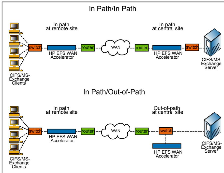
EFS WAN Accelerators are transport-level TCP proxies that conceptually operate in pair-wise configurations, with an HP EFS WAN Accelerator situated near one or more servers (the “server site”) and another situated near clients (the “client site”). Though EFS WAN Accelerators communicate with one another in a paired fashion, the architecture allows them to be clustered and meshed across the
