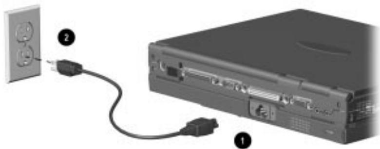
**NOTE:** Do not place anything on power cords or cables. Position them so that no one may accidentally step or trip over them. Do not pull on a cord or cable. When unplugging from the electrical outlet, grasp the cord by the plug.
