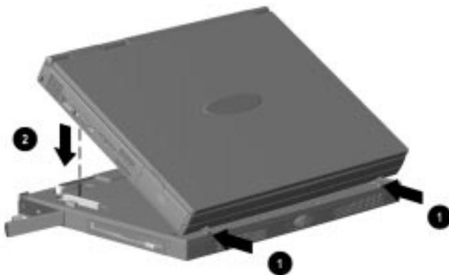
6. Push in the expansion lever to secure the computer to the M35EU.
