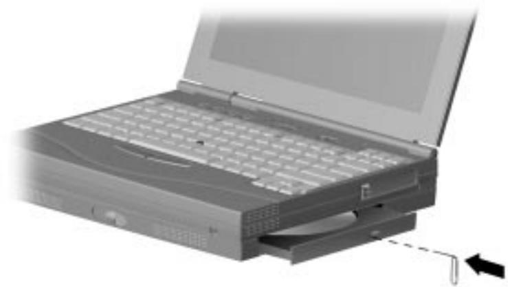
2. When the eject mechanism is released, slowly pull the loading tray out from the drive until it is fully extended, then remove the CD.
