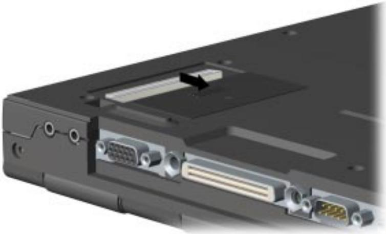
4. On the M35EU, press the expansion lever release button ❶, to release the expansion lever ❷.
