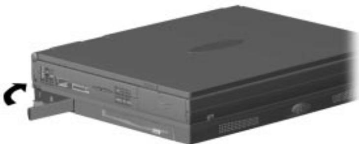
7. Slide display latches forward ❶, to open the computer ❷.
