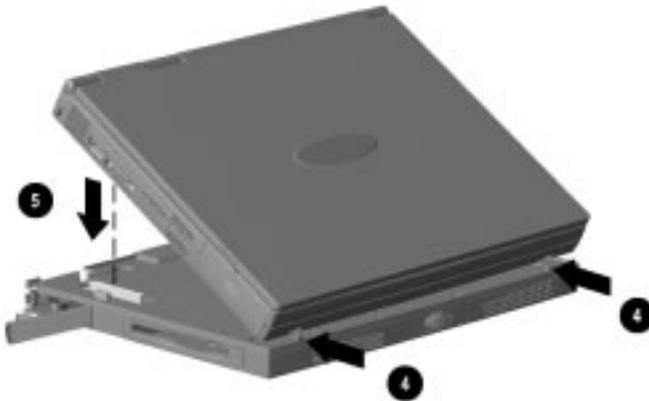
9. Push the ejection lever in to secure the computer to the M35EU.
