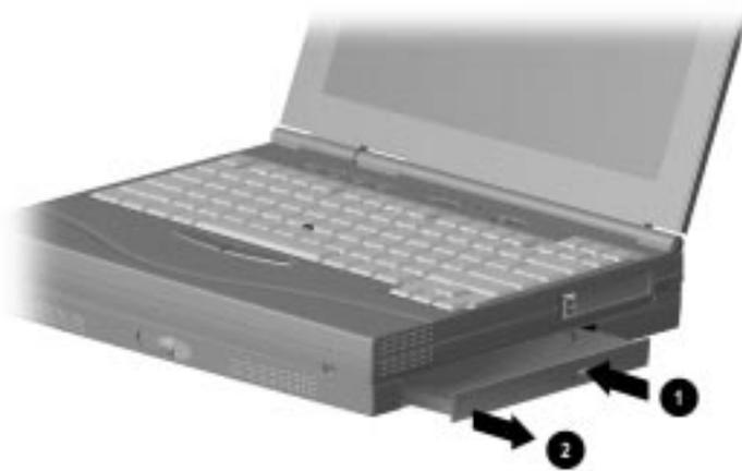
4. Remove the disc from its protective case and place it in the loading tray, label side up 3. Handle the disc by the edges, not by the flat surfaces.
