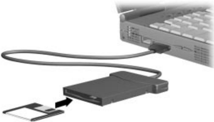
If the diskette is inserted correctly, it drops into position inside the drive and the diskette drive button pops out.
