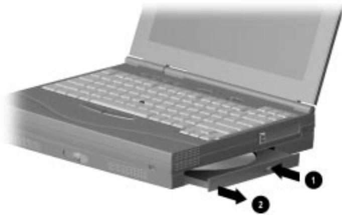
4. Remove the disc from the tray 3. Handle the disc by the edges, not by the flat surfaces.
