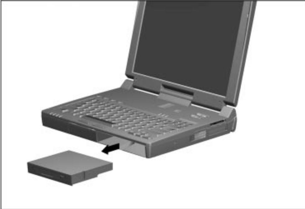
*Figure 5-24. Removing a Drive from the MultiBay*
