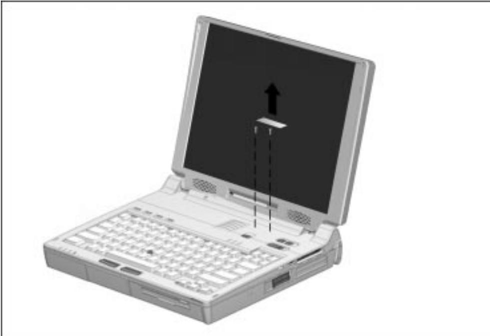
*Figure 5-31. Removing the Keyboard Warning Label and Screws*
