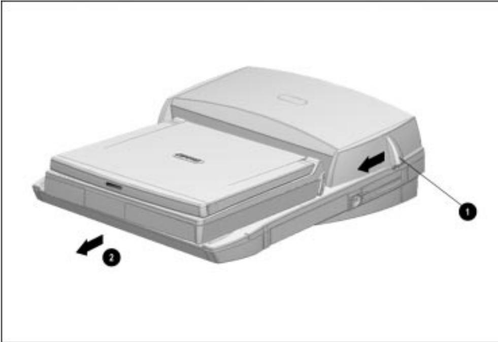
*Figure 5-5. Undocking the Computer from the Armada MiniStation*
