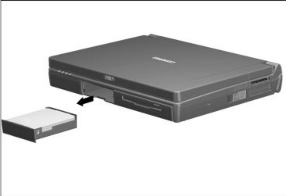
*Figure 5-16. Removing a Hard Drive from the Hard Drive Bay*
