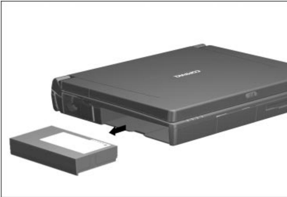
*Figure 5-10. Removing a Battery Pack from the Battery Bay*
