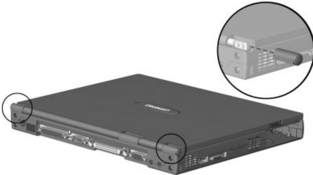
**Figure 5-16.** *Removing the Hinge Covers*
