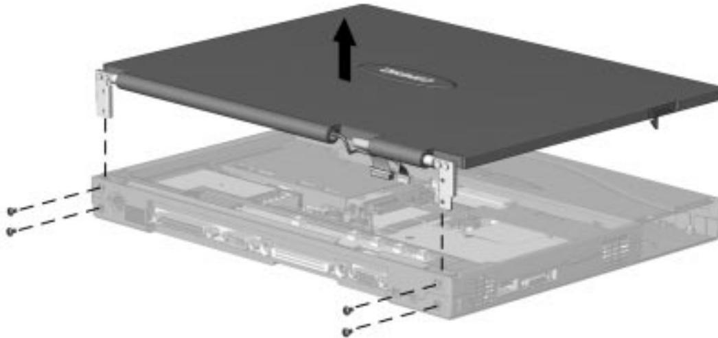
**Figure 5-20.** *Removing the Display Assembly*
