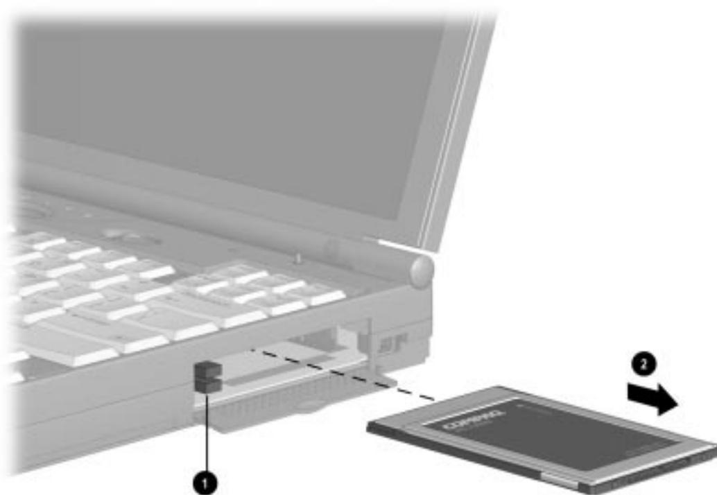
**Figure 5-5.** Removing the PC Card
