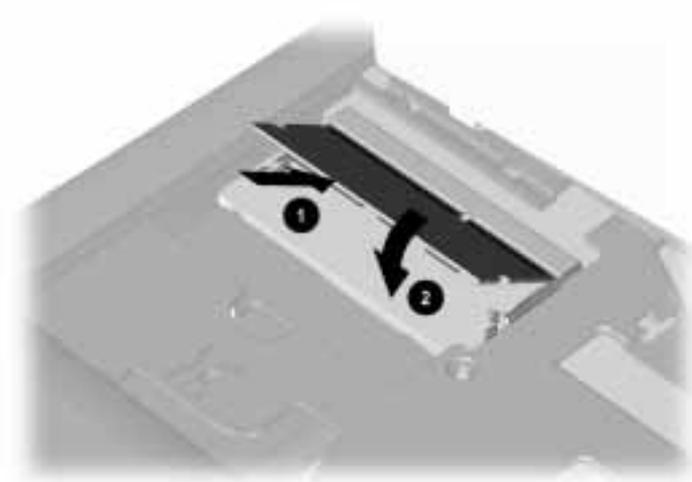
*Inserting the Memory Board*
