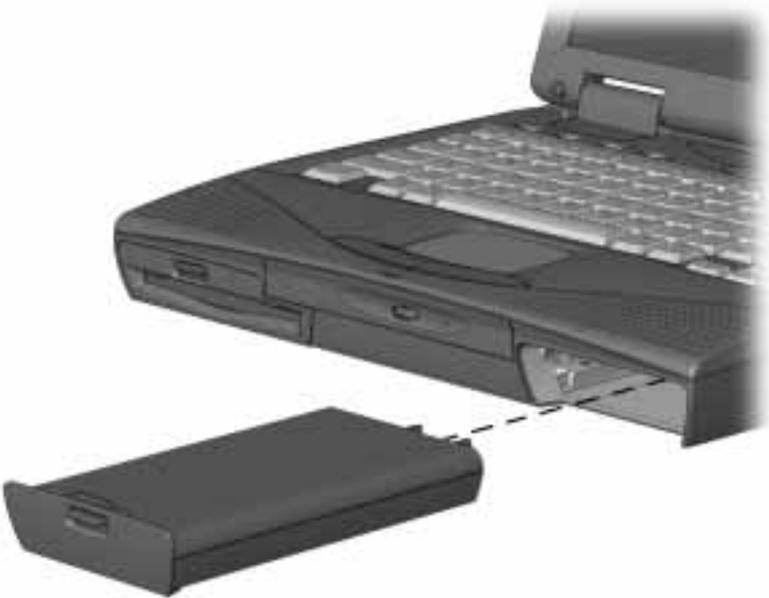
*Inserting the Battery Pack into the Battery Bay*
