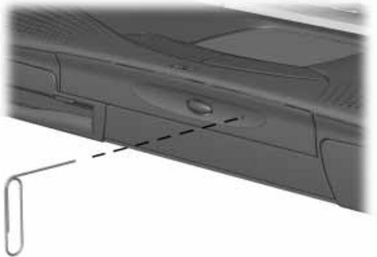
*Manually ejecting a compact disc*
