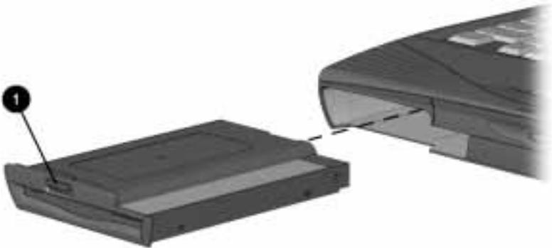
*Removing a MultiBay Device*
