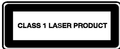
This label indicates that the product is classified as a CLASS 1 LASER PRODUCT. This label appears on a laser device installed in your product.
