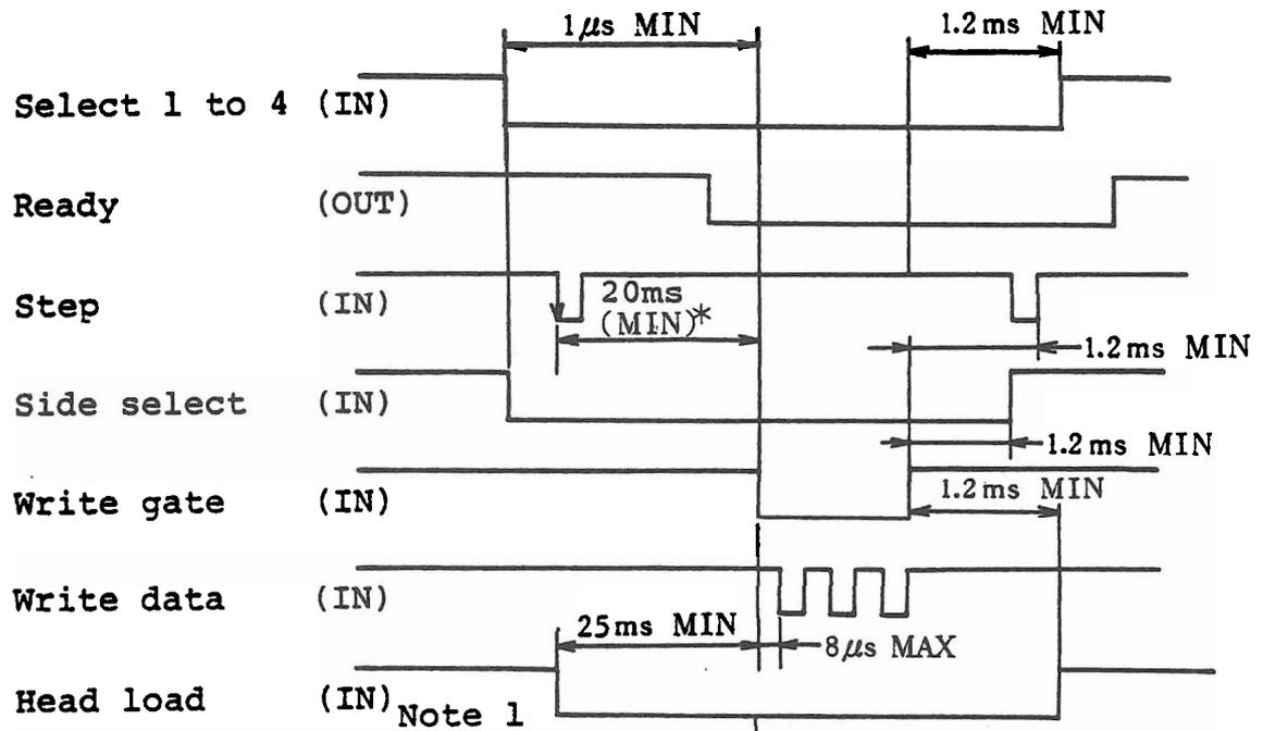
Note 1: The necessary head load waiting time is 25ms from the commencement of actual head loading.
