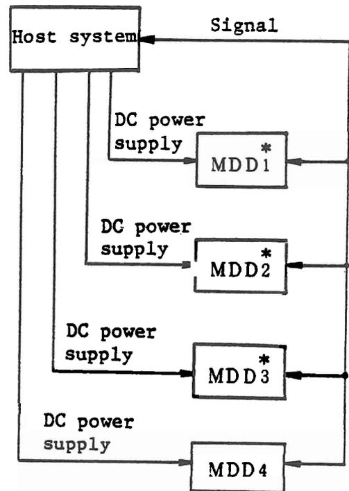
\* Remove resistor arrays.
