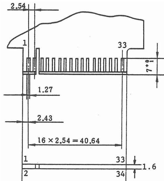
Fig. 2-1 Signal connector
