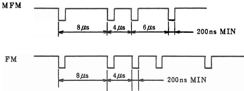
Use a write clock accuracy of  $\pm 0.5\%$  ( $4\mu\text{s} \pm 20\text{ns}$ ).
