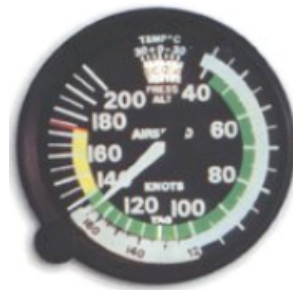
Fig. 1. Typical general aviation airspeed indicator
