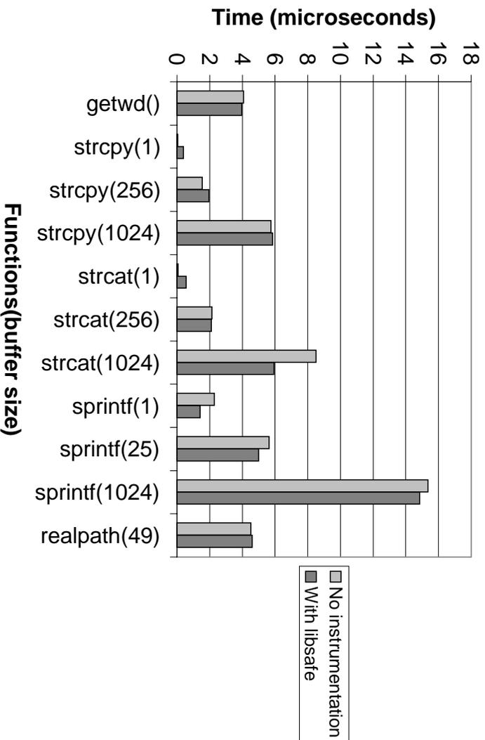
Figure 5: Performance of Libsafe Functions
