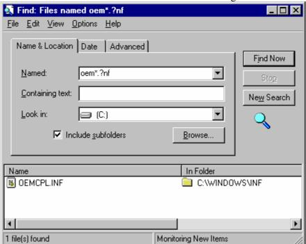
iii. Move or delete any files with names similar to those found by the previous search. If "oem1.inf" was found previously, you should delete "oem1.inf" as well as "oem1.pnf" if it exists. Do not remove "oem3.inf" simply because it appeared in this search however.
