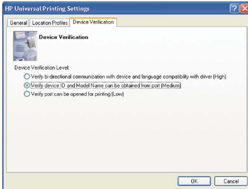
**Figure 4-3** Device Verification tab
