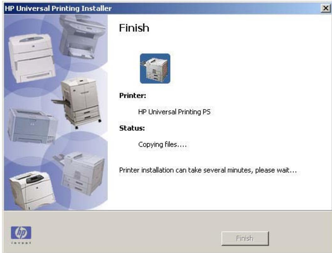
**Figure 3-15** HP Universal Printing Installer Wizard — Installing window
