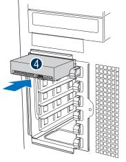
Insert fixed hard drive into drive bay until it stops. Ensure that the power and data connector end of the hard drive is facing
