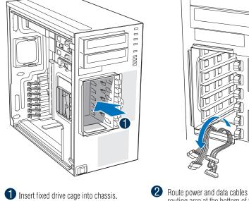
2 Route power and data cables through cable routing area at the bottom of the fixed drive cage.
