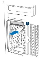
**5** Push drive latch in to lock hard drive into
