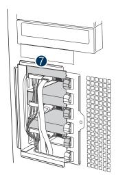
Install power and data cables to each of the installed drives. The cables route through the oval opening at the bottom of the drive cage.
