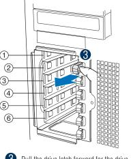
3 Pull the drive latch forward for the drive bay you want to install a hard drive in. Drive slots 1, 3, and 5 MUST be populated first. Failure to do so could result in thermal issues within chassis.
