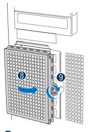
8 Re-attach drive cage EMI shield to
