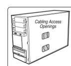
*Note: Access openings are located on the secondary side of the chassis to facilitate cable routing if necessary.*
