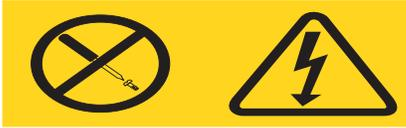
Hazardous voltage, current, and energy levels are present inside any component that has this label attached. There are no serviceable parts inside these components. If you suspect a problem with one of these parts, contact a service technician.
