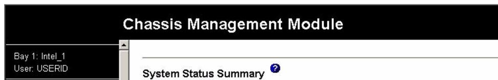
The upper-left corner of the management module Web-interface page shows the login ID of the current user and the location and identity of the active (primary) management module. In the preceding examples, the login ID is USER1, and the primary management module is identified as SN#01 and is installed in management module bay 1.
