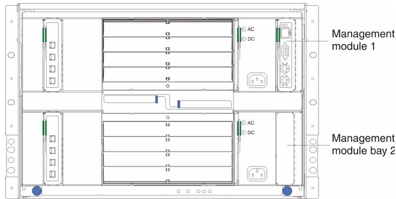
**Attention:** To maintain proper system cooling, each module bay must contain either a module or a filler module; each blade bay must contain either a blade or a filler blade.
