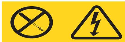
Hazardous voltage, current, and energy levels are present inside any component that has this label attached. There are no serviceable parts inside these components. If you suspect a problem with one of these parts, contact a service technician.
