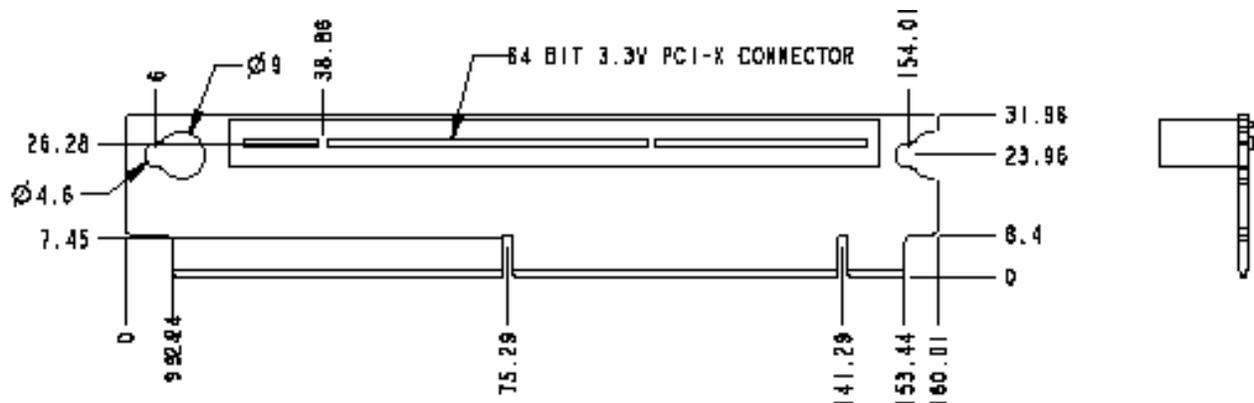
Figure 40. 1U Full-Height PCI-X Riser Card Mechanical Drawing
