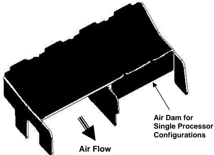
Figure 19. CPU Air Duct
