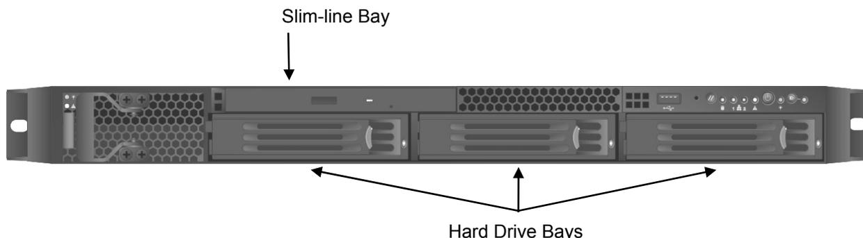
Figure 22. Intel® Server Chassis SR1450 Peripheral Bay Configuration Options
