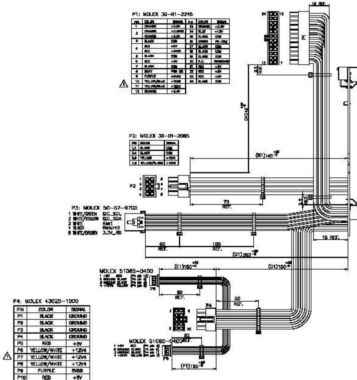
Figure 12. Power Distribution Board Harness Detail
