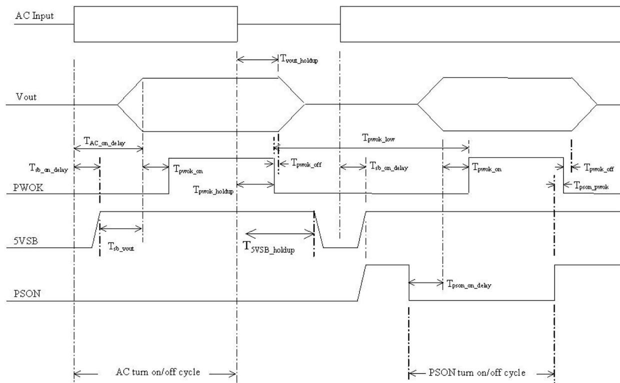
Figure 14. Turn On/Off Timing (Power Supply Signals)
