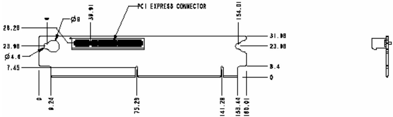
Figure 41. 1U Full-Height PCI-Express Riser Card Mechanical Drawing
