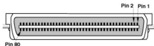
Figure 31. 80-pin SCA2 SCSI Interface
