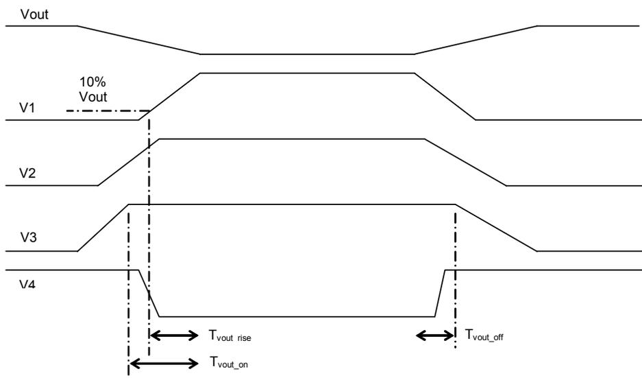
Figure 13. Output Voltage Timing
