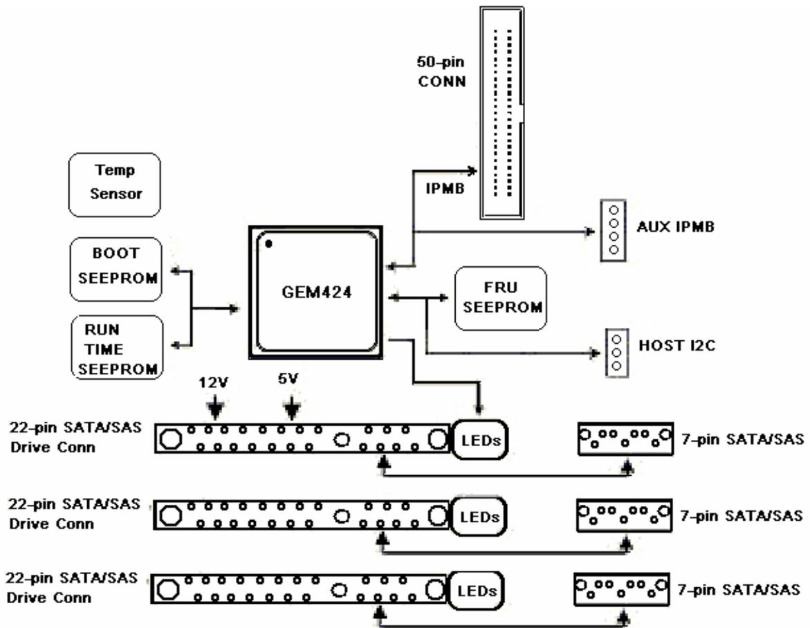
Figure 33. SATA/SAS Backplane Functional Block Diagram
