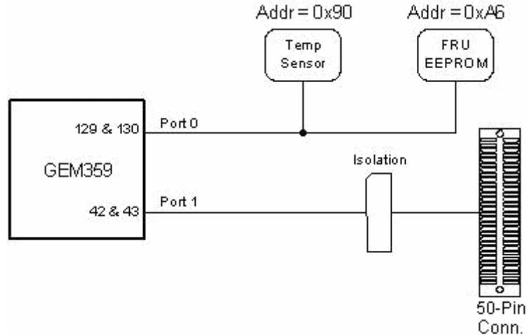
Figure 29. Intel® Server Chassis SR1450 1U SCSI HSBP I2C Bus Connection Diagram
