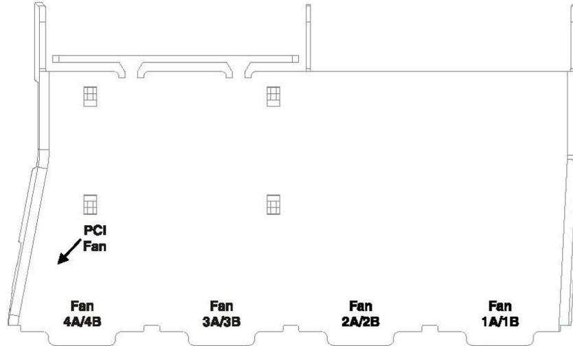
Figure 20. CPU Air Duct Fan Numbering
