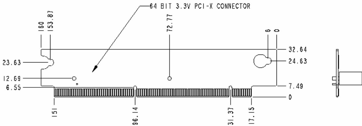
Figure 42. 1U Low-Profile PCI-X Riser Card Mechanical Drawing
