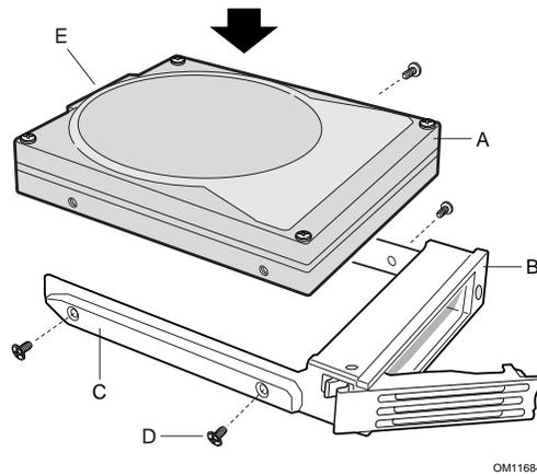
**Figure 25. Hard Drive Tray Assembly**
