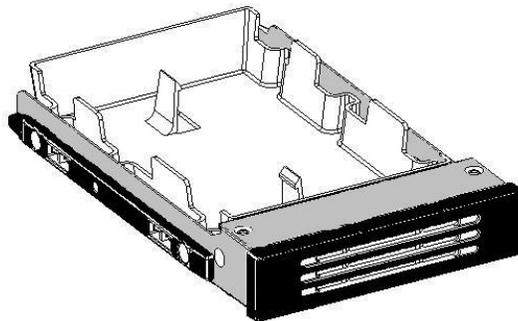
**Figure 26. Drive Tray with Drive Blank**
