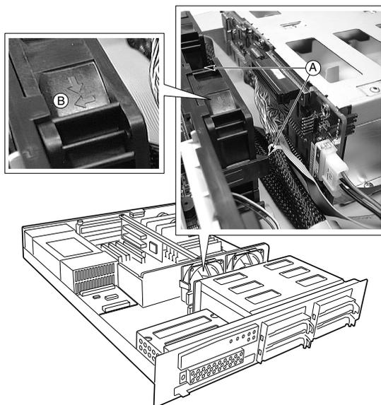
**Figure 50. Replacing a Fan**
