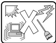
The system is designed to operate in a typical office environment. Choose a site that is:
