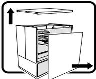
After you have completed the six SAFETY steps above, you can remove the system covers. To do this:
