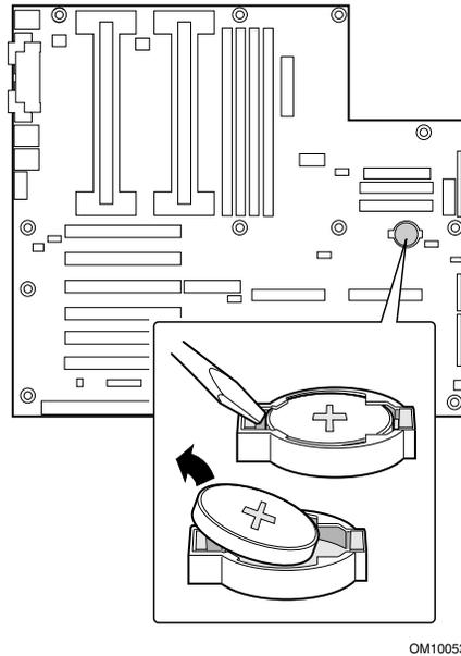
**Figure 54. Replacing the Server Board Battery**
