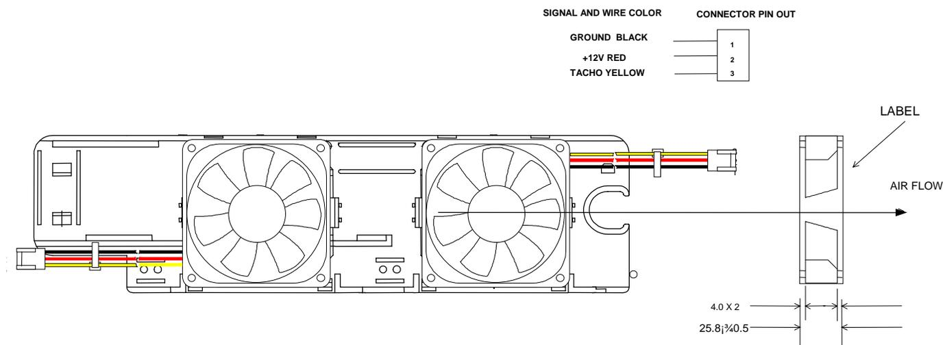
Figure 6. 80mm Mid System Fan
