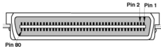
Figure 12. 80 Pin SCA2 Connector
