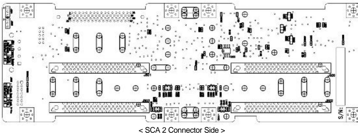
Figure 9. SR2000 Hot-Swap SCSI Backplane Component and Connector Placement
