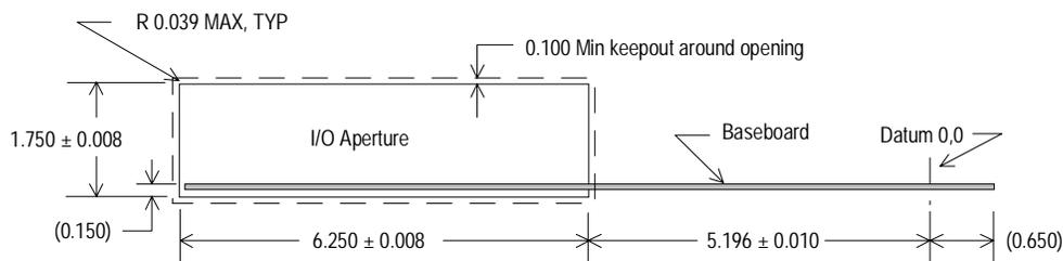
Figure 4. ATX 2.03 I/O Aperture
