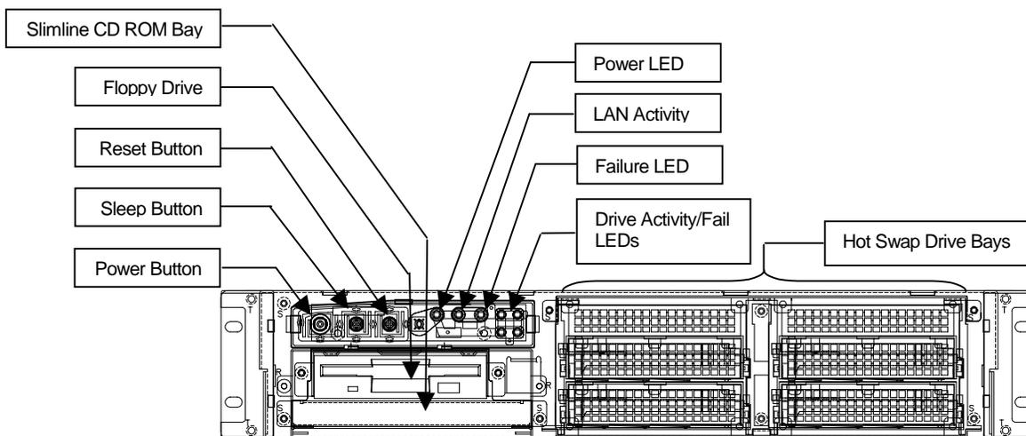
Figure 2. Front View of SR2000 without Front Bezel
